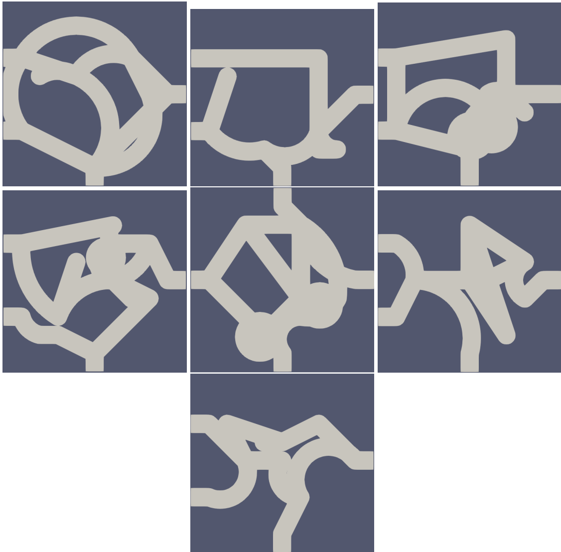
Figure 6.10: Potential diode-like 4-port devices found by KMeans with no preprocessing.
