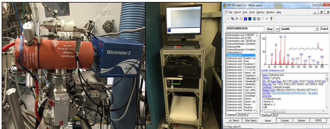
Figure 57. MKS Microvision 2 quadrupole mass spec tool in ANSLab with control computer rack and screenshot of compound fragmentation software used to identify  $q/m$  peaks.
