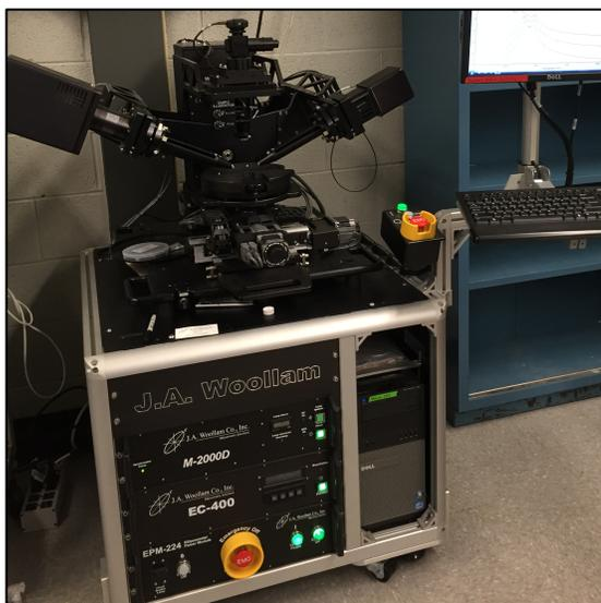
*Figure 60. J.A. Woollam M-2000D spectroscopic ellipsometer used for measuring optical properties of thin films. This image shows the ellipsometer on its base, however the source and detector can be mounted to the Ultratech Fiji F-200 ALD tool for in-situ sensing.*
