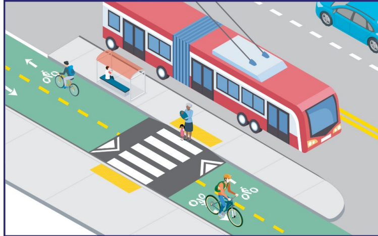
Fig. 2.7 "Two-way protected cycle track with a wide raised crossing to a transit island." (Opfell & DeLuca, 2019)
