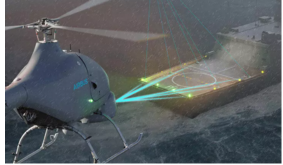
(b) Position localization using RF ranging signals.
