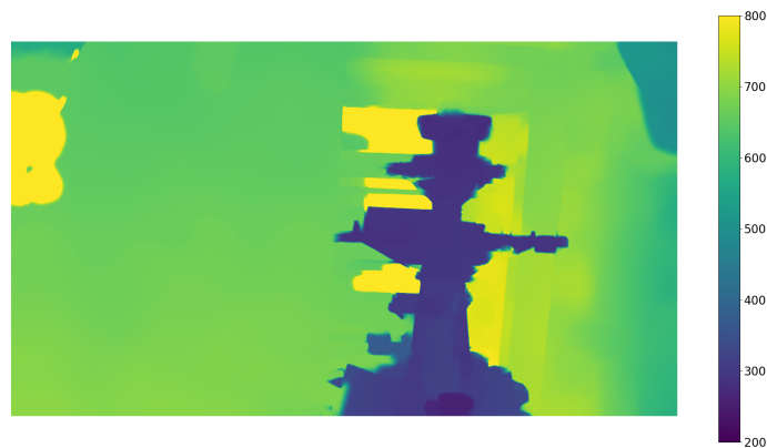
(b) The depth map used to remove the image background. The depth map provides an estimated distance from the camera in millimeters for each pixel in the image.
