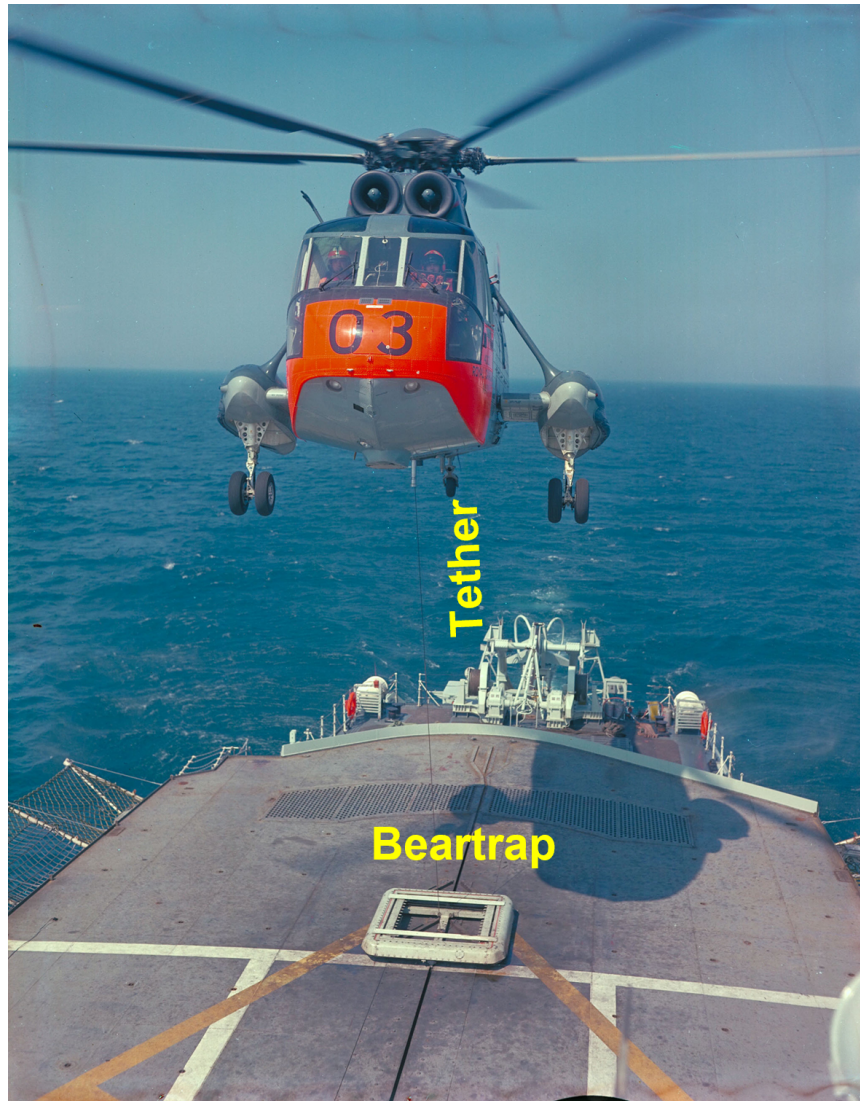
Figure 1.4: On May 25, 1967, Sea King helicopter CH-SS2 is hauled down by a Bear Trap to a landing on the deck of Her Majesty's Canadian Ship Assiniboine. (Courtesy Department of National Defence / PCN-67-415)
