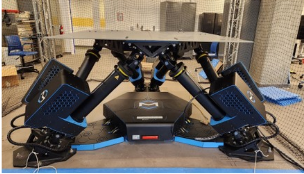
Figure 6.1: Large Stewart platform with attached 6×6 foot fiberglass surface to be used for vision-based autonomous landing. The platform can recreate severe sea states up to Sea-State 7.
