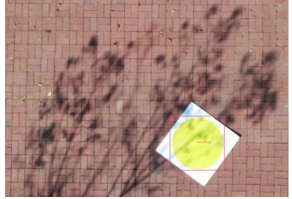
(b) Detection of landing marker using neural network [27].
