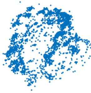
(b) A 3D point cloud showing the positions of features detected on the object. This result is produced using several dataset images.
