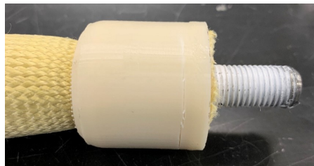
Figure 16: End-fitting Socket delamination
