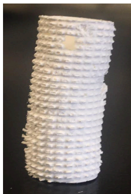
Figure 3.2. Alumina membrane green body from NMP/PVB/Alumina slurry. The slurry resulted in better filling which in turn led to better shape retention of the mold. However, there are large holes, surface defects, and slight tilt.
