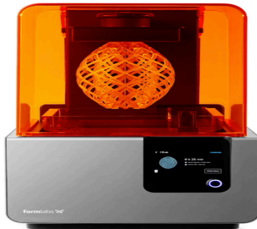
Figure 2.6. An image of the Form2, which has a build volume of 145x145x175mm. It is Formlabs' second-generation desktop printer and was used to print the designs presented in this study. 16
