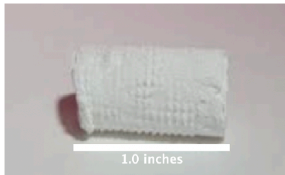
Figure 2.13. Isolated alumina green body after completing phase-inversion via immersion precipitation and demolding.
