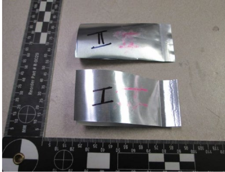
Figure 12 Sample I and sample II prepared for measuring the seal strength using the tensile testing machine
