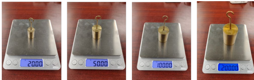
Figure 62 Picture showing the calibration of weighing scale used in the experiments
