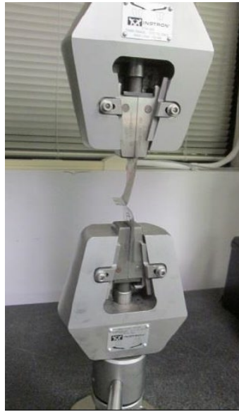
Figure 14 Picture showing the MBB samples that are being clamped onto the grips of the tensile testing machine
