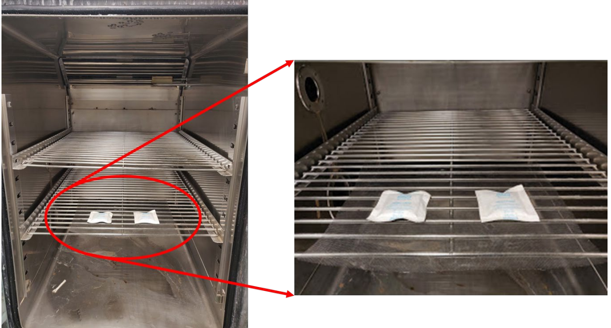
Figure 17 Representation of desiccants placed inside the temperature/relative humidity chamber
