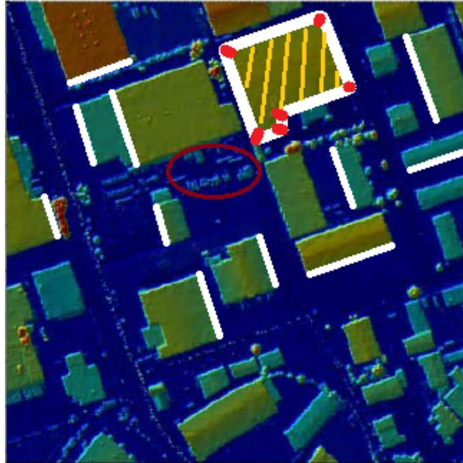
This image, figure 2.28 is as urban as DEM tiles get. The buildings have flat or slightly sloped rooves, the buildings align on a grid that appears to be shifted approximately 20 degrees. There are very few details (circled) to stand in the way of large simple objects to represent.
