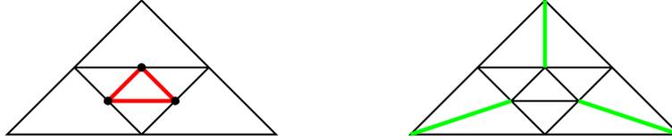
Figure 7.2: Regular refinement. Left: red refinement and hanging nodes; Right: green closure.
