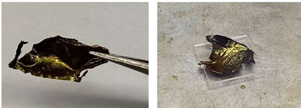
Figure S7.82. Image of free-standing metallic luster film of (+)PMCP-PBI-(+)PMCP:P3HT blend (1:1 by mass).
