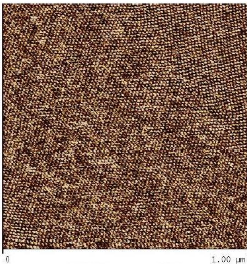
Figure S5.14. ps-tm AFM phase map of a 60-nm-thick film of aPMP- b -PCL, VIII on a c-Si substrate annealed at 100 °C. For all materials in this study please see †.
