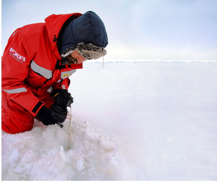
Figure 6.6: The author collecting ice thickness measurements during MOSAiC. A standard thickness gauge was used in all measurements (photo by: Laura Wischniewski).
