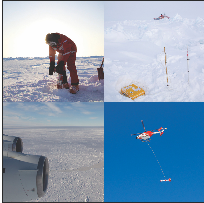
Figure 1.5: Sea ice thickness measurement techniques. Clockwise from top left: manual drillings (photo by: Laura Wischnewski), automated thermistor buoys (photo by: Steven Fons), airbourne (helicopter) EM soundings (photo by: Steven Fons), and airborne (fixed-wing) laser/radar instruments (photo by: Jeremy Harbeck).
