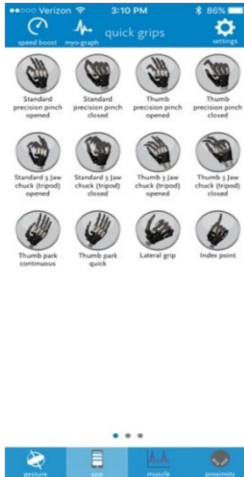
Figure 2.3 My i-limb grip selection screenshot (Touch Bionics, Apple App Store, 2020) (Figure modified from Figure 1 of Wang et al., 2022[95])
