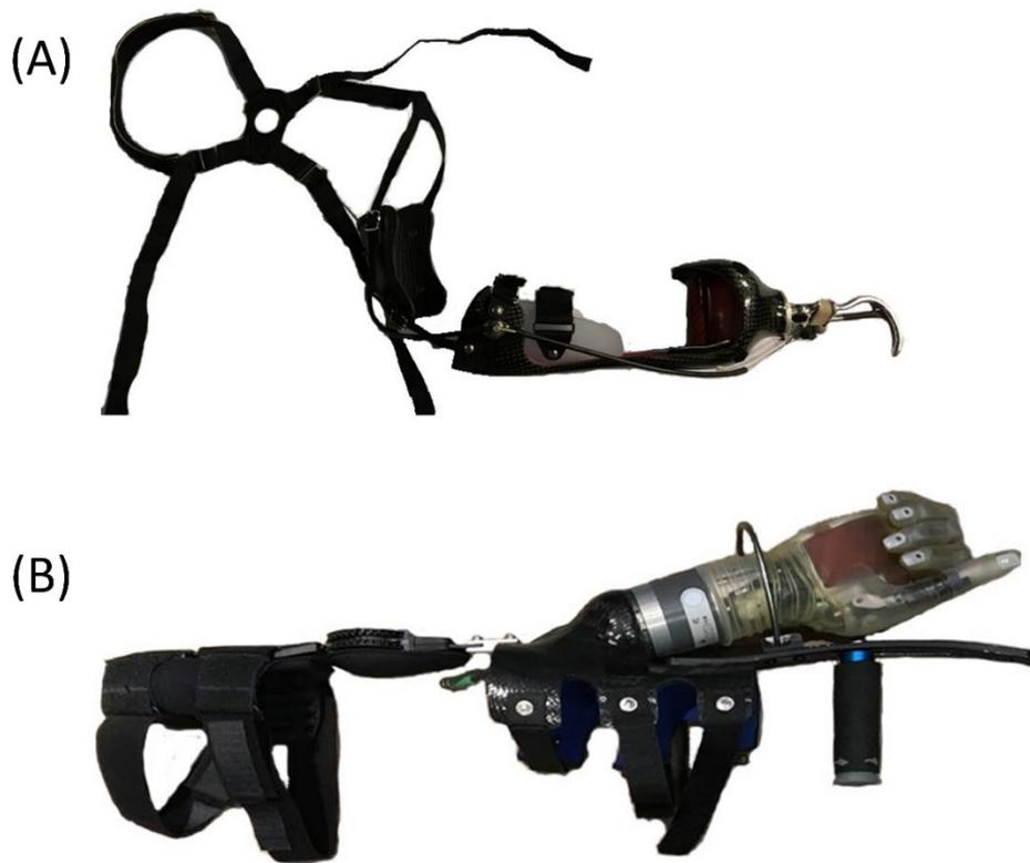
Figure 3.1 Upper limb prosthesis bypass devices. A) Body Powered Bypass device, right side configuration with body-powered voluntary open Hosmer 5x split hook terminal device. B) DEKA Bypass device, right-hand radial configuration with powered wrist. (Figure 1 of Wang et al., 2021[93])
