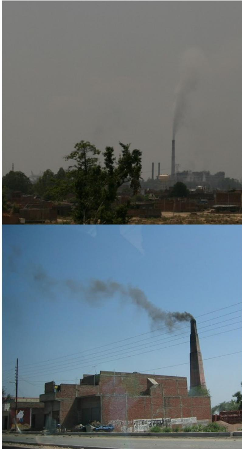
**Figure 2.3 Fossil fuel aerosol sources, such as the coal-fired Panki power plant (top panel) and a coal-fired mix of agricultural waste and/or wood in a Bull's Trench kiln (bottom panel), emit black carbon particles and precursor gases (e.g. nitrogen oxides and sulfur dioxide) to form nitrates and sulfates contributing to aerosol loading in the atmosphere over Kanpur, India.**
