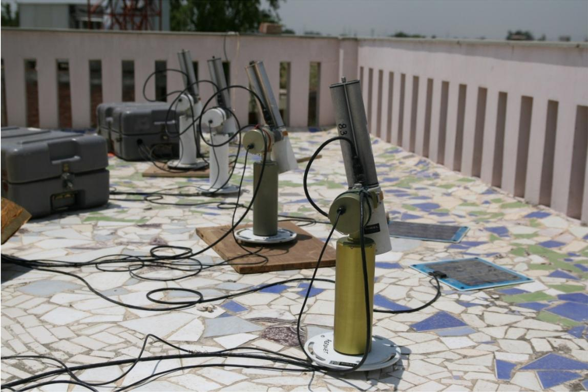
**Figure 1.1 Cimel Sun/sky Radiometers deployed in Kanpur, India. Using a robot controlled by azimuth and zenith motors, the instrument points directly at the Sun given the time, location, and aid of a 4-quadrant detector. Light passes through a collimator tube, sensor head lens, and wavelength-dependent transmission filter on a filter wheel until it reaches a Silicon or InGaAs detector inside the sensor head canister. Photo courtesy of Sheng-Hsiang Wang.**
