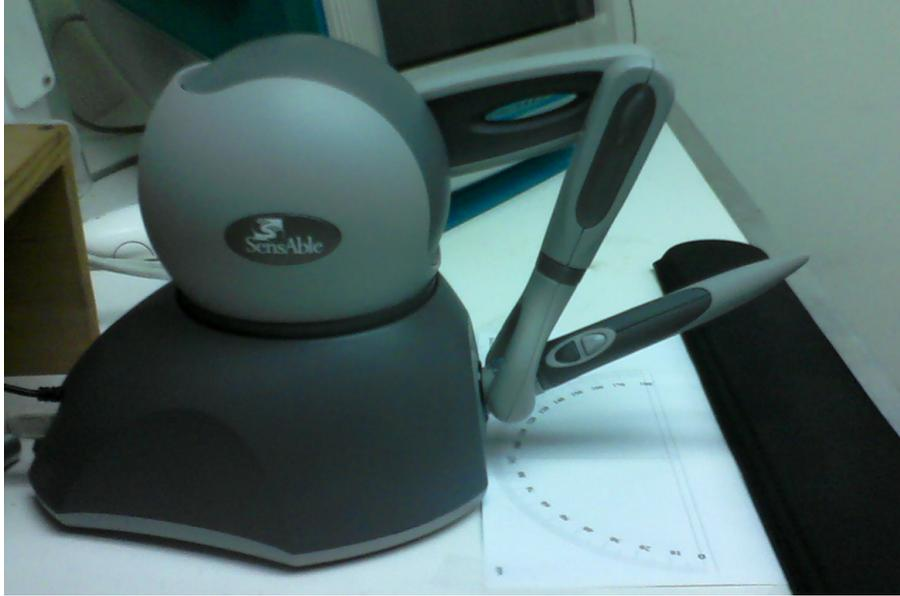
Figure 5.1: Setup of the Phantom Omni device with gel wrist support and reference protractor.
