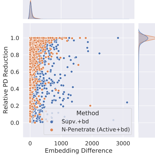
Figure 4.7: We plot the joint distribution of relative PD reduction ( Y -axis) and embedding difference ( X -axis) over successfully collision-handled test meshes in the SCAPE dataset for our method and Supv+bd . Our method resolves more collisions (average PD reduction 94.81% vs. 88.76%) while remaining closer to the input (average embedding difference 56.17 vs. 66.11) as compared with Supv+bd .
