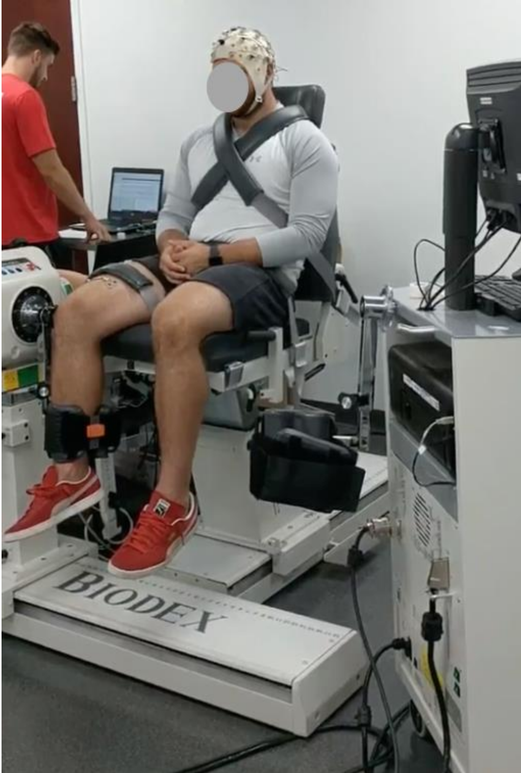
Figure 3.3. The experimental set-up demonstrating a participant engaging in an experimental strategy while seated on the isokinetic dynamometer (Biodex® System 4 Pro).
