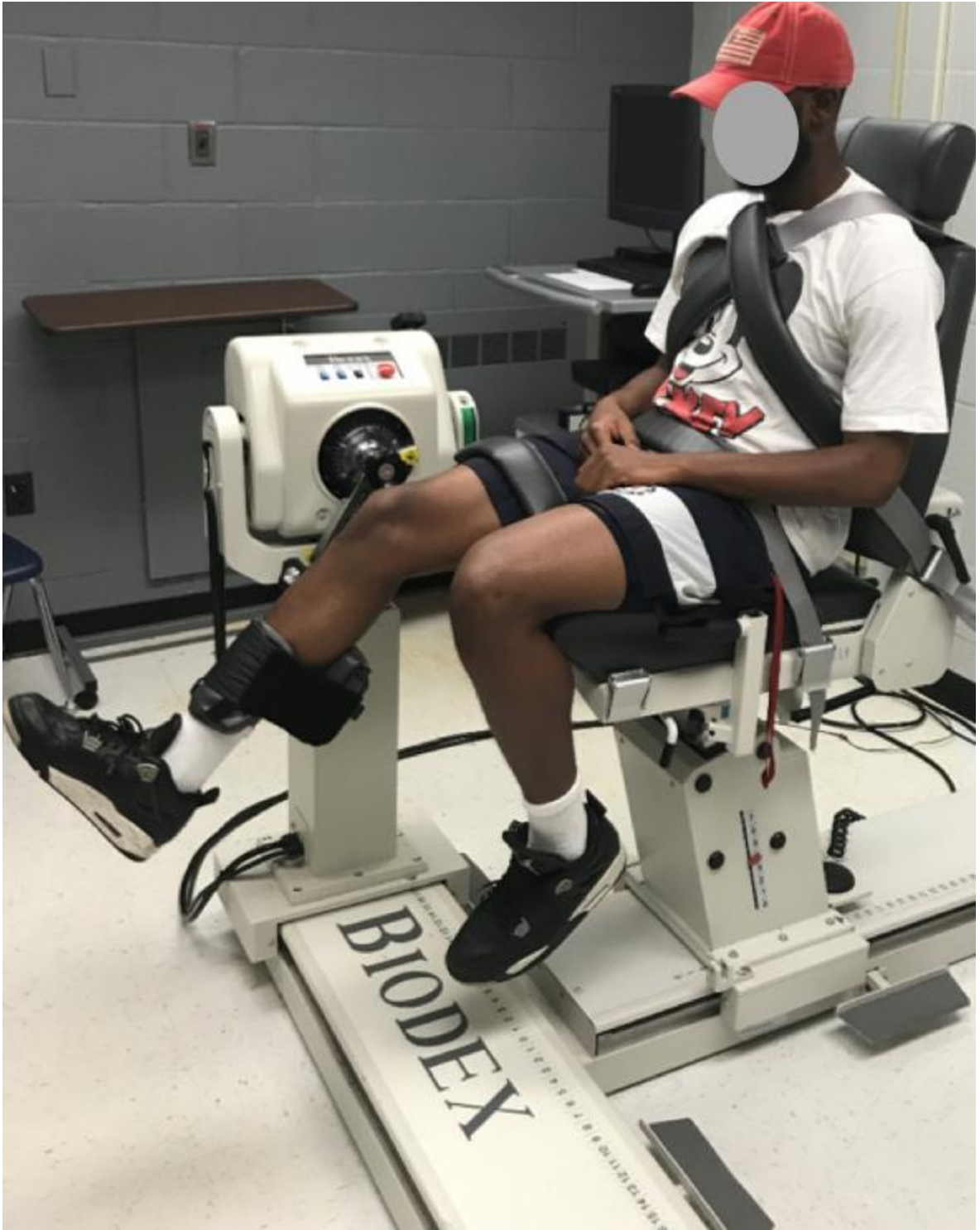
Figure 2.1. The experimental set-up demonstrating a participant engaging in an experimental strategy while seated on the isokinetic dynamometer (Biodex® System 4 Pro).
