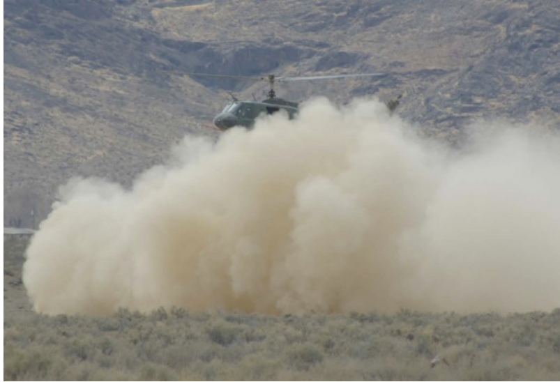
Figure 1.1: A helicopter encountering brownout conditions during a landing. (Photo is courtesy of Optical Air Data Systems LLC.)
