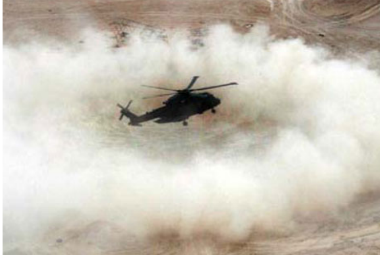
Figure 1.2: A landing helicopter with the formation of a more favorable ring or toroidal shaped dust cloud that forms away from the immediate landing zone.
