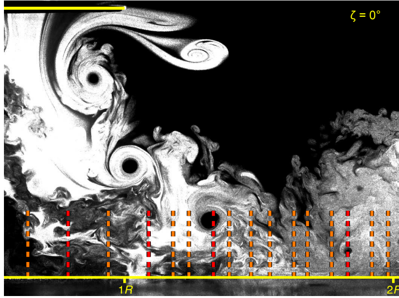
(a) A FV image capturing the rotor blade parallel to the light sheet ( \Delta\zeta = 0 ).
