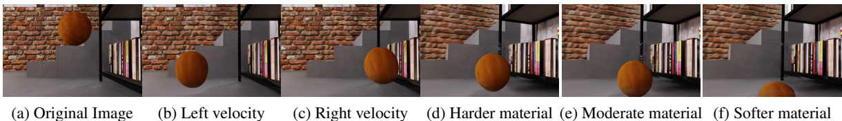
Figure 6.6: Parameter estimation and editing by differentiable physics. NeuPhysics can estimate the acceleration and Young’s Modulus, generate new videos with different initial velocities and material parameters.
