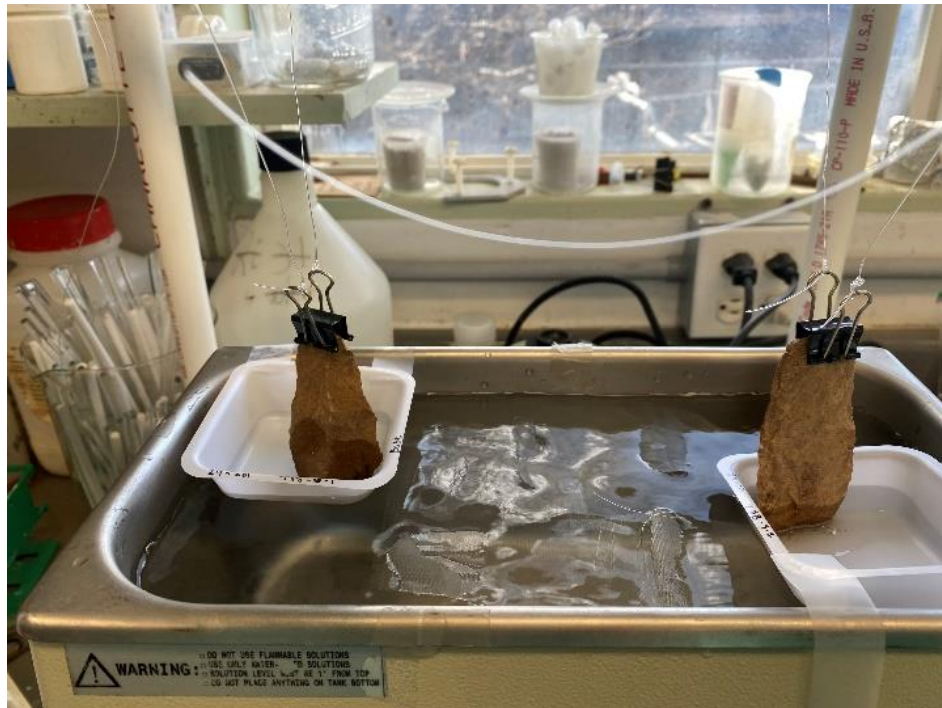
Figure 4 Ultrasonic bath for bases of artifacts (Used with permission from Michael Stork)
