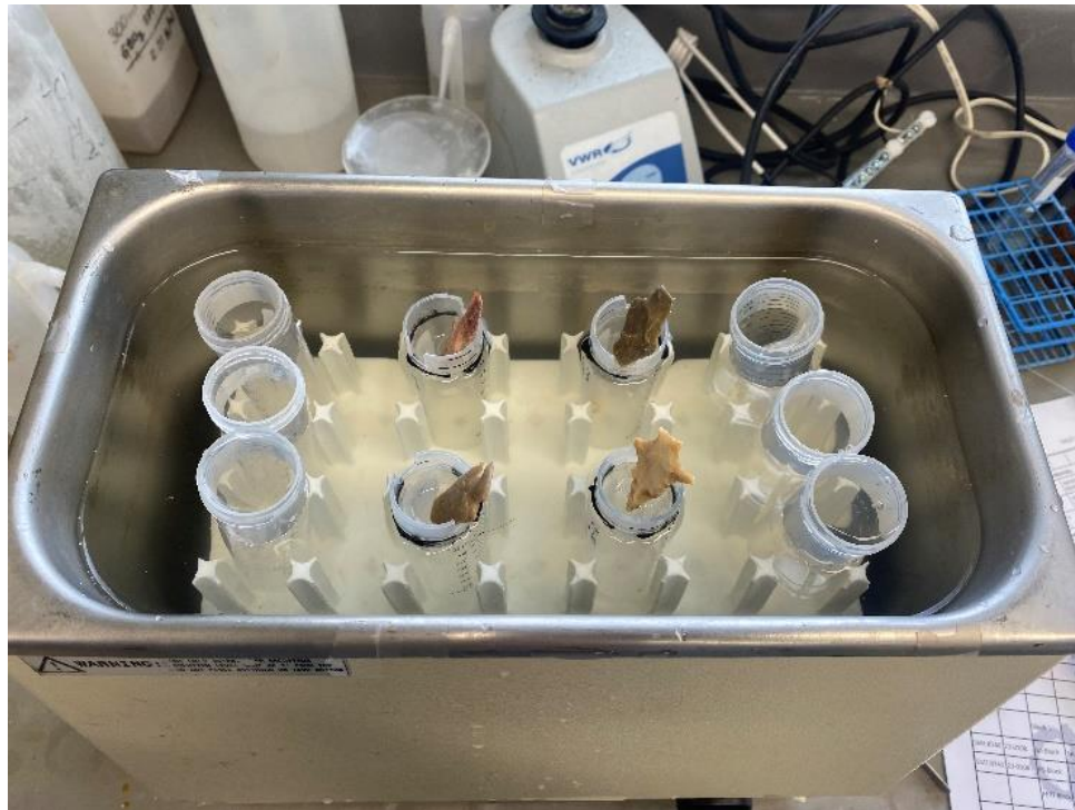
Figure 5 Ultrasonic bath for tips of artifacts (Used with permission from Michael Stork)
