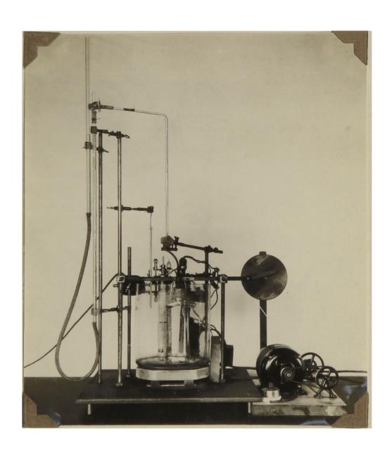
water temperature is equalized by a motor-driven stirrer of the turbine type. The Bunzel tube is shaken at the rate of approximately 204 complete excursions per minute and the thermostat kept constant at  $24.5 \pm {}^{\circ}\text{C}$ . In starting the shaker motor, the switch is thrown one second before the minute which allows the first mixture to occur approximately on the minute. Readings are taken at the end of each successive minute for periods of 3, 5, or 10 minutes.
