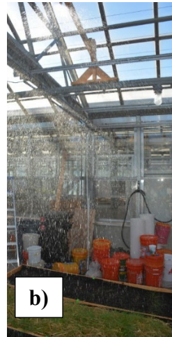
Figure 4-7: (a) Rainfall simulator with a single jet nozzle to produce synthetic rainfall which produced surface runoff collected in (b) sample bottles at the base of the slope. (c) the cross-sectional view of the runoff setup. Runoff was captured in the gutter system for collection and analysis with a rain guard to protect the effluent from dilution due to applied rainfall.
