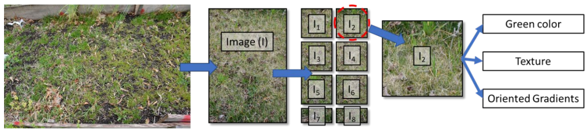
Figure 4-8: Flow chart of (left to right) the original image captured, cropping to the region of interest, segmentation into pixel blocks, and extractions of feature descriptors for algorithm input.
