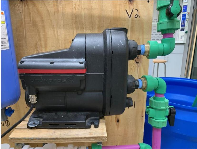
**Figure 3C:** Grundfos SCALA2 Pump.
