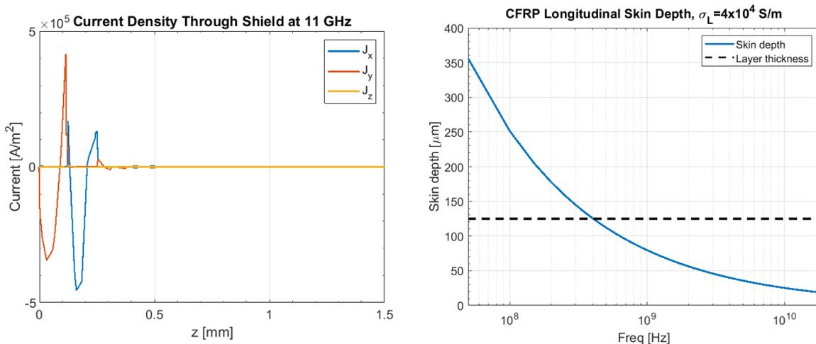
Figure 7.15.A) Current density x, y, and z components through the shield in the z-direction at 11 GHz. The layer thickness is 0.125 mm. Current flow changes direction within a single ply, however the skin effect, where the induced current should be confined to the surface of the ply, is not accurately reflected by the model. B) Plot of skin depth vs. frequency indicating that at 11 GHz the skin depth should be smaller than the ply thickness.
