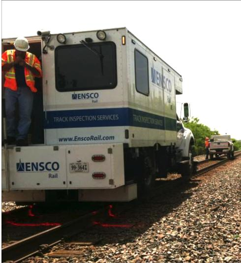
Figure 4.4: CTIV platform used to collect the images.
