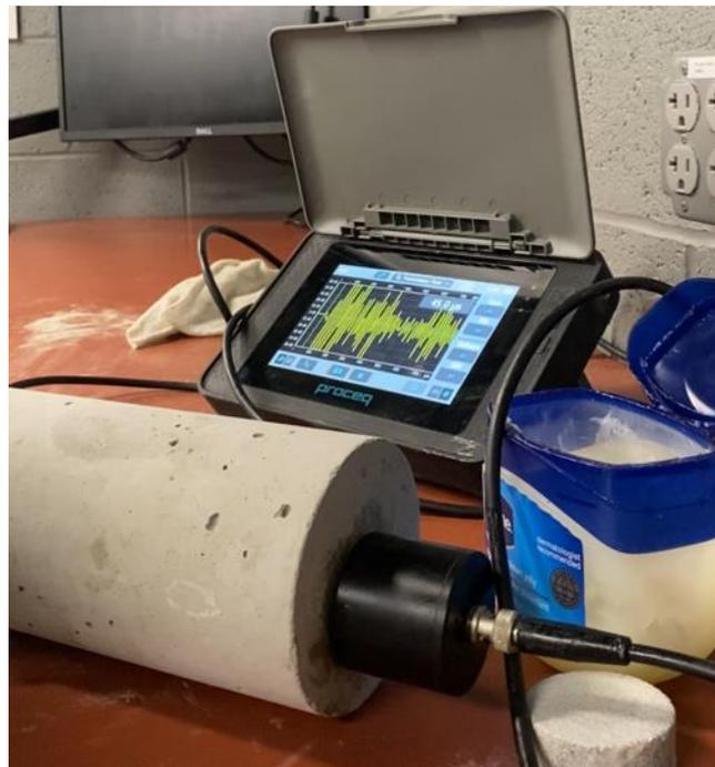
**Figure 2.2. Ultrasonic pulse velocity (UPV) testing setup**
