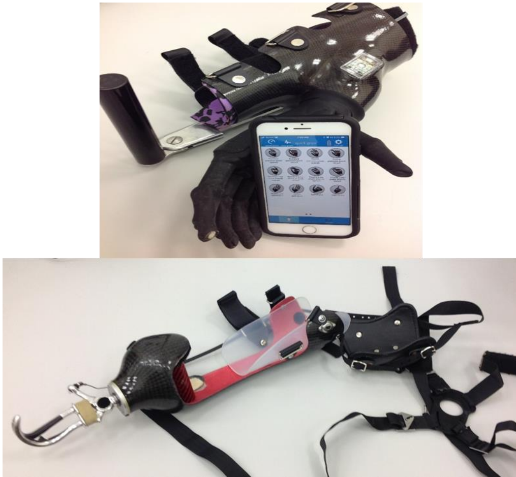
Fig. 1. i-limb® Ultra Myoelectric Bypass Prosthesis with Biosim smartphone application(top picture). Body-powered bypass prosthesis with voluntary opening Hosmer 5X hook (bottom picture).
