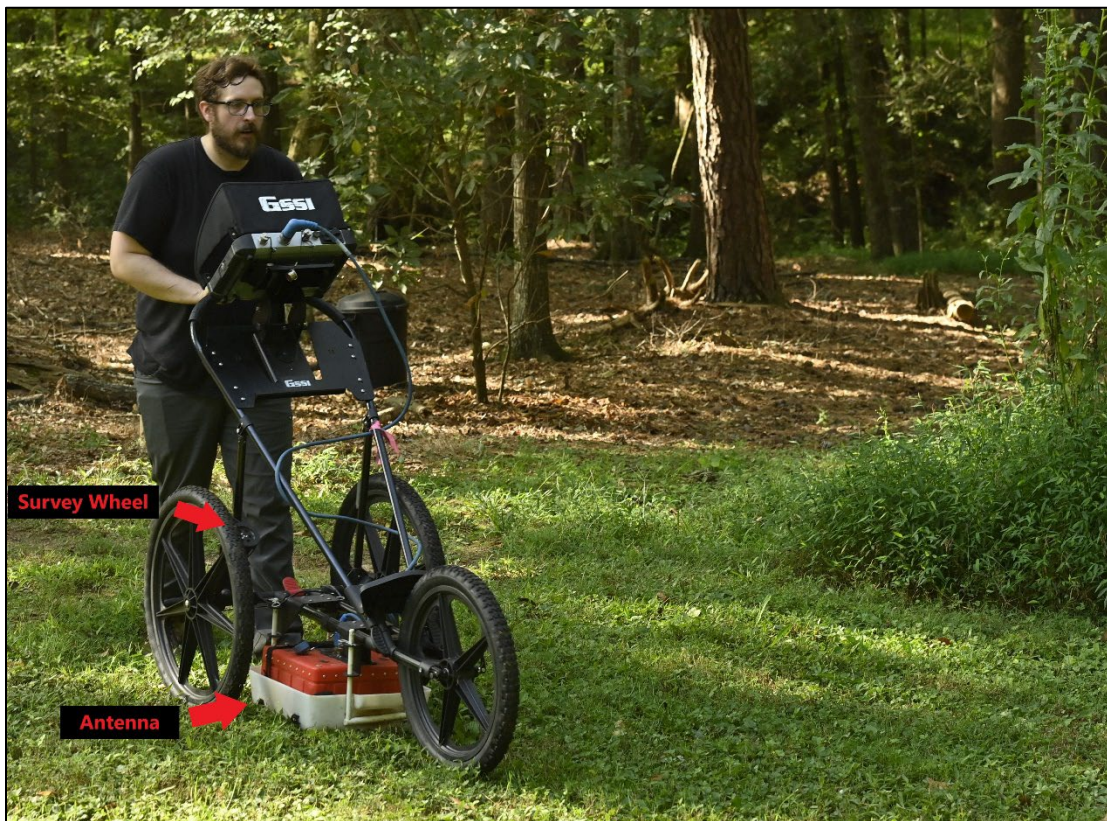
Figure 2.1. GPR setup with receiving antenna pushed along the ground by a three-wheel cart with an attached survey wheel (Photo courtesy of Georgia Gwinnett College).
