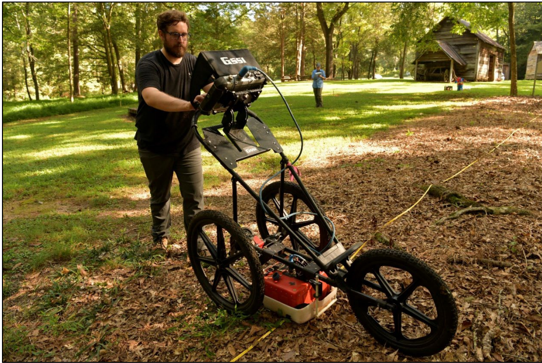
Figure 1.3. Conducting the second GPR investigation at site 9WN168 (Photo courtesy of Georgia Gwinnett College).
