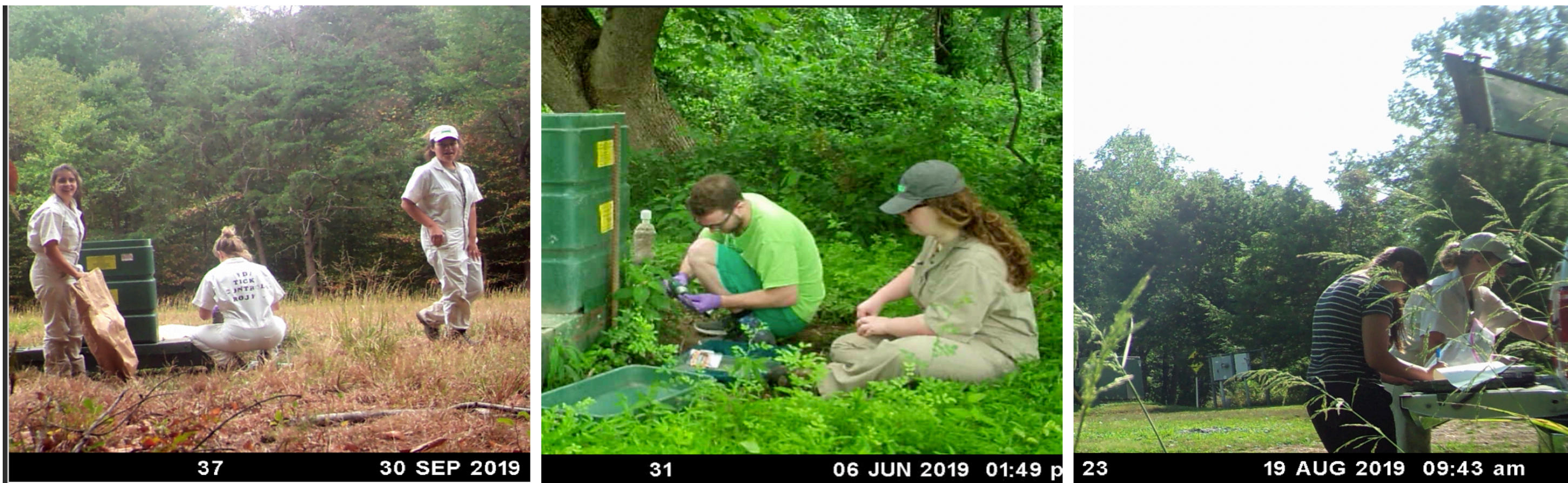
Figure 9. Examples of maintenance work for the "4-Poster" devices. From left to right, maintenance work includes refilling the device with bait, reapplying permethrin to rollers, removing clogs and molding corn bait, and recording how much corn bait was consumed.
