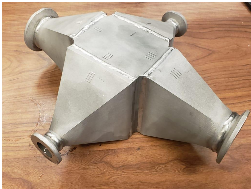
Figure 6-17: Fabricated headers and flanges (a) cold side (b) hot side
