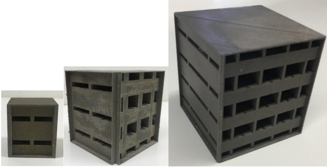
Figure 4-15: Image of the (a) 1"×1"×1", (b) 2"×2"×2", (c) 3"×3"×3" M2HX unit fabricated out of maraging steel
