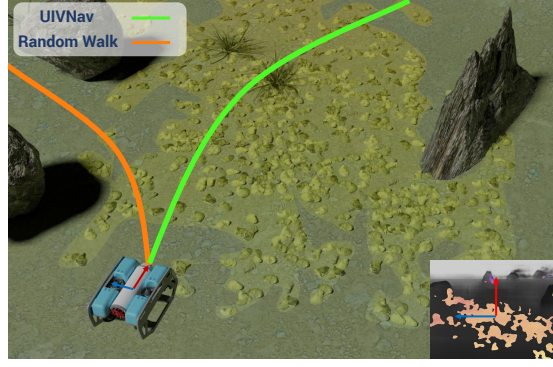
Figure 3.3: Example of BlueROV surveying reef of oysters in simulation (translucent mask is applied on the oyster reef for better visualization.)
