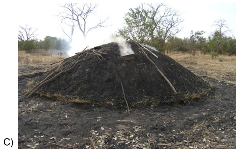
Figure 1-2 - Steps in charcoal production. A) Collection of fuel for carbonization; B) Piling of wood into kiln structure; C) Lit kiln actively carbonizing wood; D) Removal of charcoal from outside of kiln.
