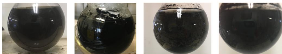
Figure 5-3. From left to right, pH-adjusted GO nanofluids after boiling and condensation experiment for 0 days (as prepared), 1 day, 2 days, and 3 days.
