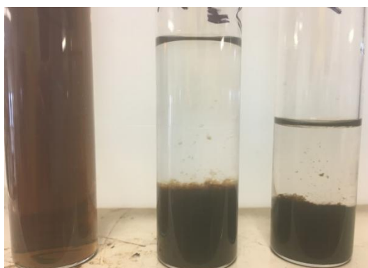
Figure 5-2. From left to right, GO nanofluids prepared with pH = 4.8 (as prepared), pH = 2.4, pH = 12.5.
