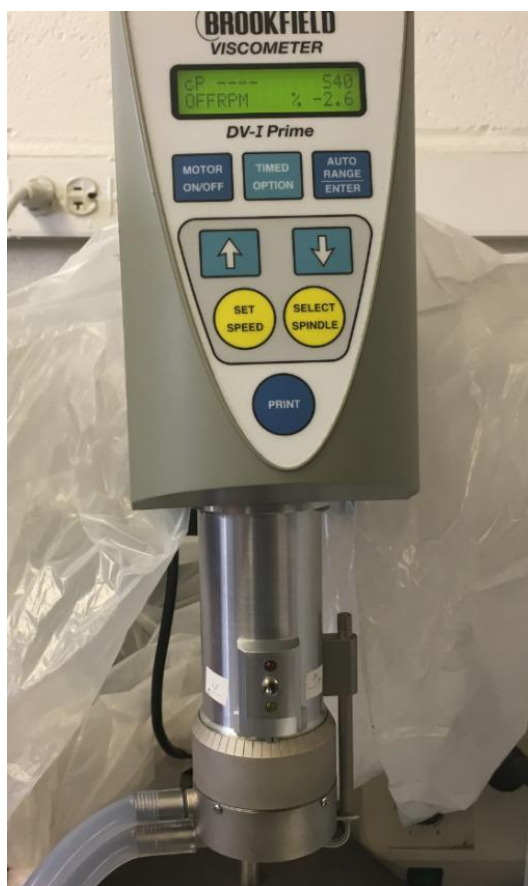
Figure 3-1. Viscometer (Brookfield DV-I Prime) used for the viscosity measurement.
