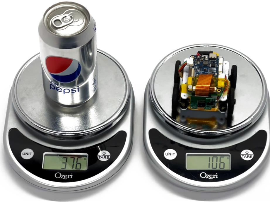
Figure 1.10: Weight comparison between a 330ml of Pepsi can with the tiny autonomous car.
