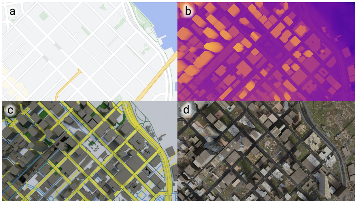
Figure 4.4: (a) OpenStreetView, (b) Depth Map, (c) 3D Model View Generated by WorldGen and (d) Final Rendered View
