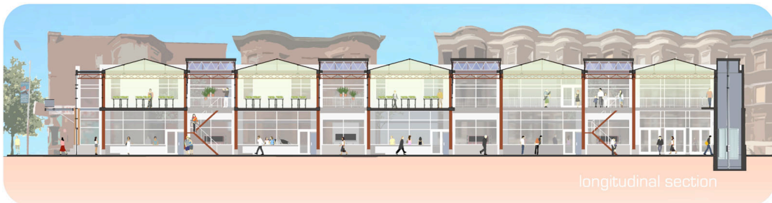
Figure 39 – Longitudinal section through greenhouses and market aisle
