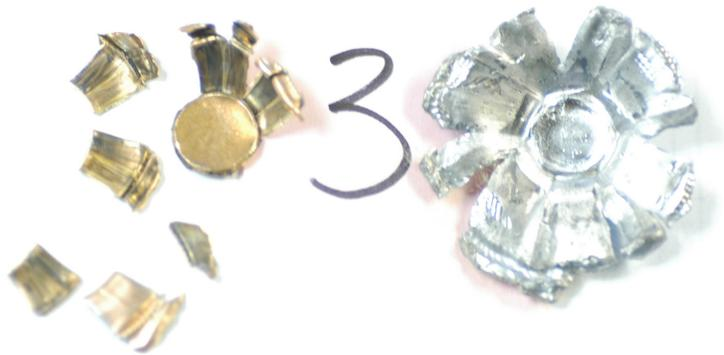
Figure A.18: Photograph of shattered bullet removed from armor.
