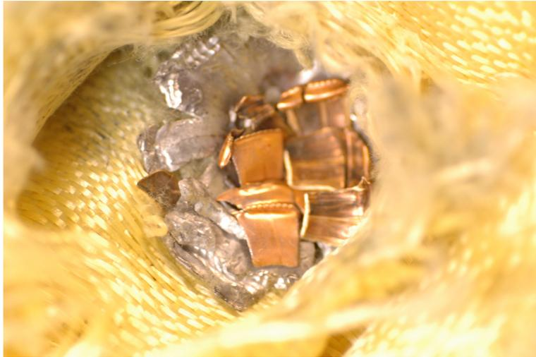
Figure A.17: Photograph of de-constructed armor with shattered bullet inside.
