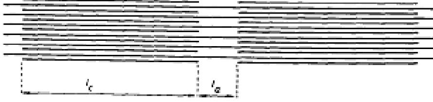
Figure 4.6: Schematic model of the gel-spun hot-drawn UHMPWE fiber, consisting of crystal blocks with length  $l_c$  and disordered domains with length  $l_a$  [115].
