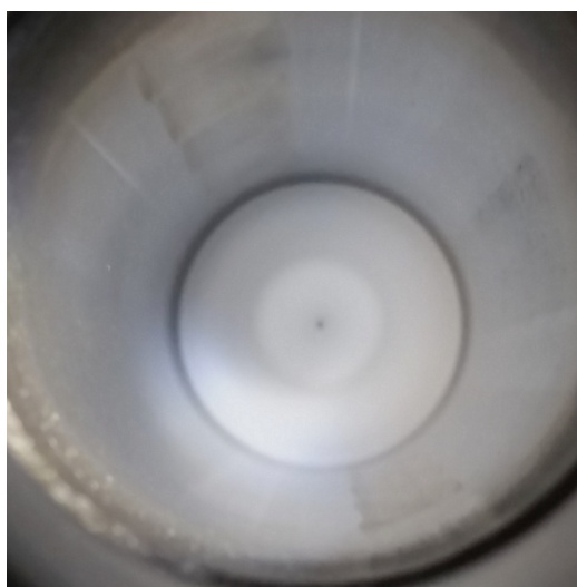
(b) Fully clogged trap
