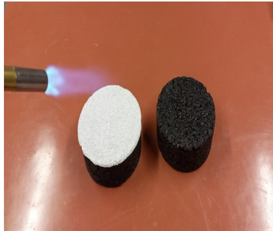
Figure 2.2: Application of Preformed Thermoplastic on asphalt surfaces
