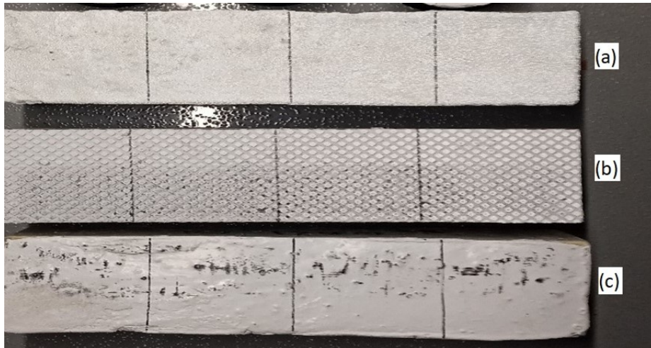
Figure 3.4: Pavement Markings: (a) Preformed Thermoplastic, (b) High-Performance Tape, (c) Thermoplastic
