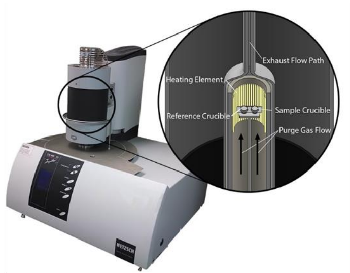
Figure 7-1. Schematic of the Simultaneous Thermal Analysis (STA) apparatus.
