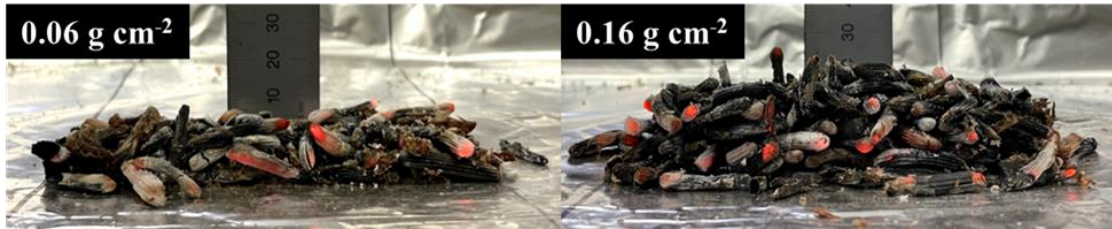
Figure 2-6. Height, in millimeters, of the two firebrand pile coverage densities positioned within the 50 cm 2 deposition area.
