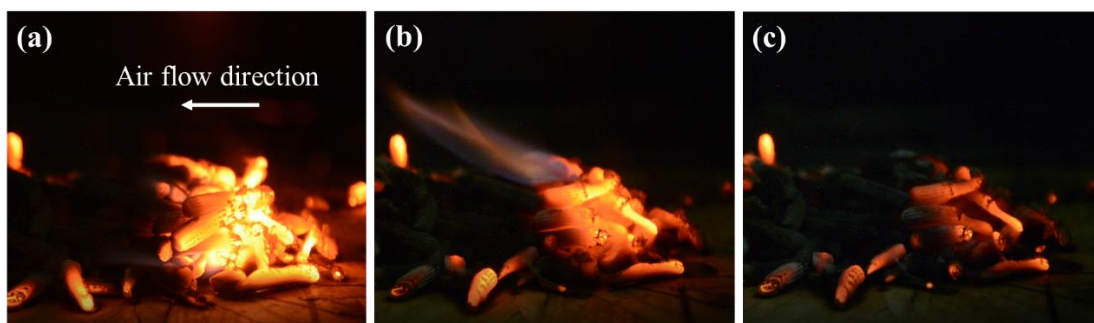
Figure 6-4. Firebrand pile glowing color differences during (a) the application of a forced air flow and (b), and (c) when the forced air flow into the wind tunnel has been terminated.
