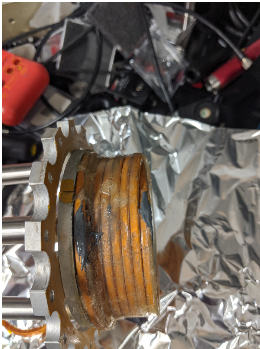
Figure 3.1: The MOT coil with epoxy applied to the two leak locations
