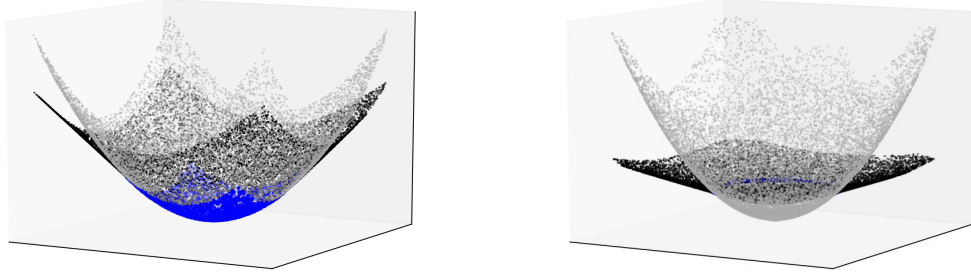
Figure 7.1: (Quadratic function) . Both panels show the learned v.s. true y = x_1^2 + x_2^2 . In each figure, we color OOD predictions by MLPs in black, underlying function in grey, and in-distribution predictions in blue. The support of training distribution is a square (cube) for the top panel, and is a circle (sphere) for the bottom panel.
