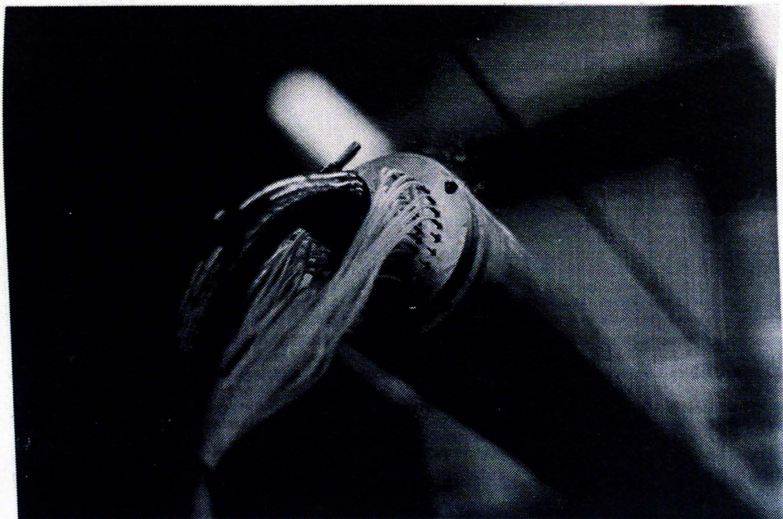
Figure 8 Air Supply Plenum and Pressure Tap Connection of the Model
