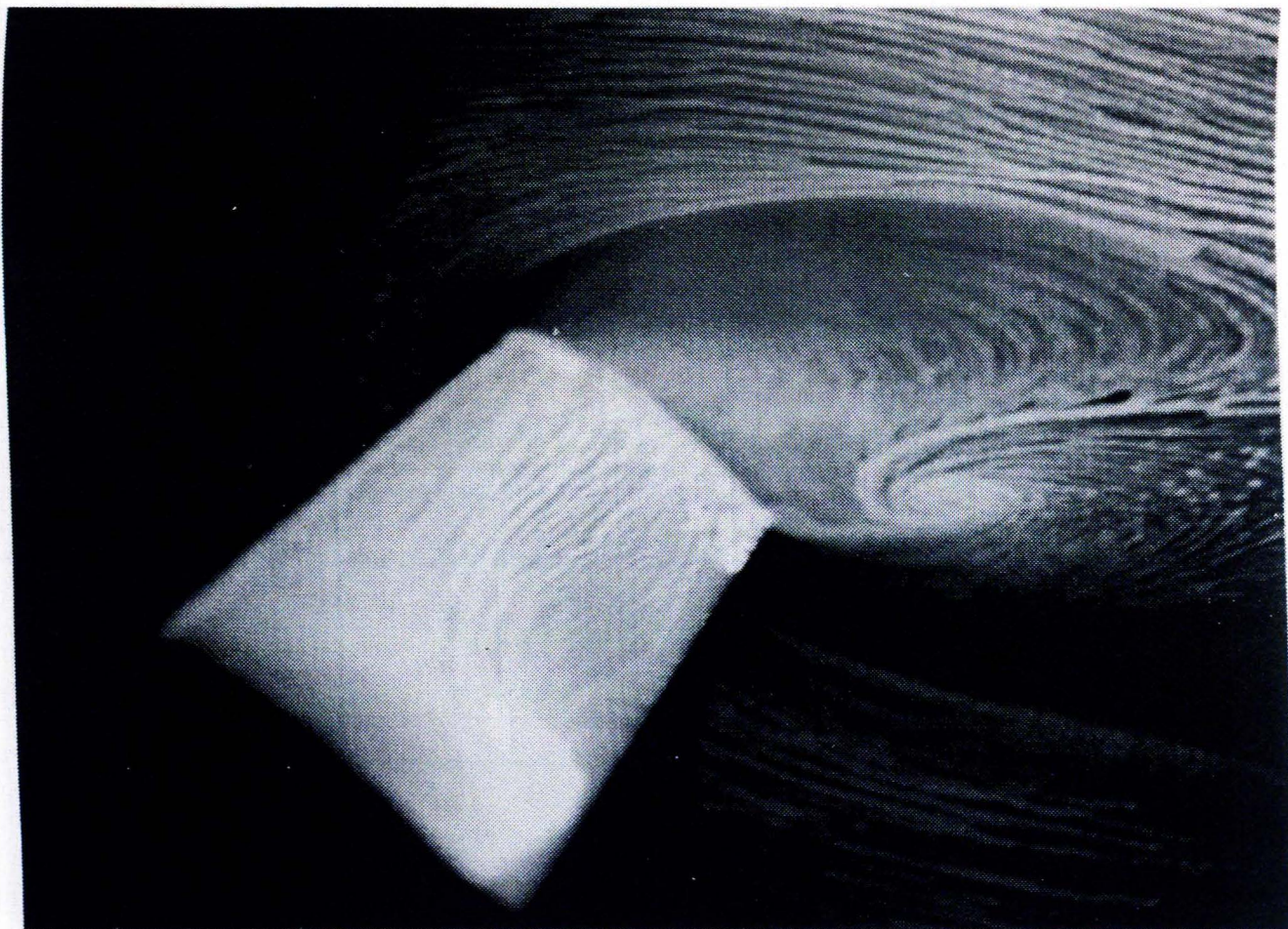
Figure 48 The Surface Oil Flow of a Wing-Wall Interaction at a High Angle Attack
