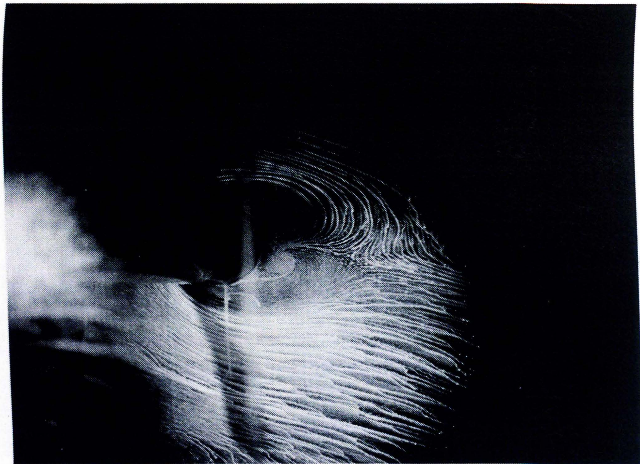
Figure 47 Oil Flow Patterns on the End Plate of the Circulation Control Cylinder with C_{\mu} = .09
