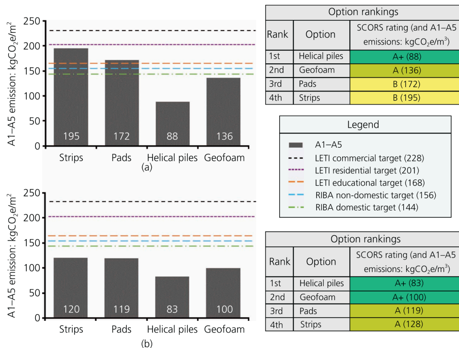
Fig. 2.28: Ranking and comparing the four design options (source: Hamza et al., 2023)
