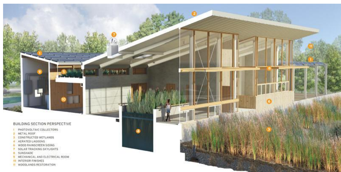
Figure 9 - Living Machine at The Living Building (Omega Institute) Source: AIATopTen.org
