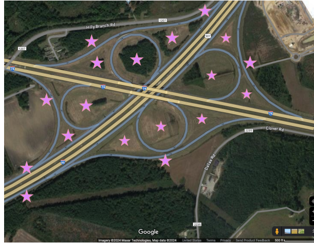
Figure 5.14: Satellite imagery from the intersection of I95 and I74. Stars indicate possible locations of ground stations. In these locations the lawn by the highway is mowed, indicating there is access to the site. Image credit in bottom of image.
