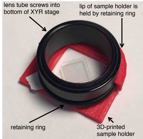
Figure 6.3: A 3D-printed sample mount holds (22\text{ mm})^2 cover slips (the substrates for our samples) and is held by a lens tube with a retaining ring. When the lens tube is screwed into the underside of the XYR stage, the sample can be translated, rotated, and quickly removed by loosening the retaining ring. The small crystal in the center is a (1\text{ cm})^2 birefringent crystal attached to the cover slip.
