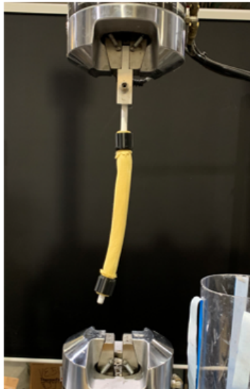
Figure 4.7: Free contraction burst test setup.
