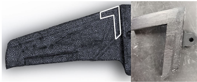
Figure 5.1: Left: Scan of v900 wing with highlighted section used for the wing holder. Right: 3D-printed wing holder with attached gear.
