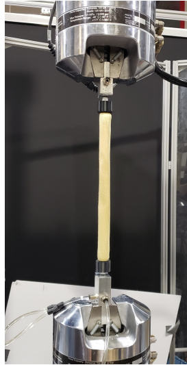
Figure 4.6: Blocked force burst test setup.
