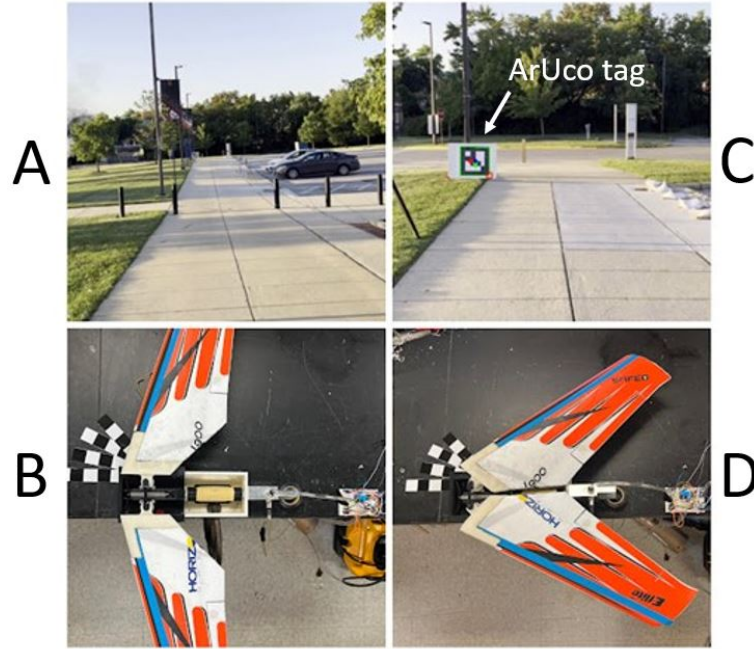
Figure 5.10: Left: No object detected in (A), resulting in no sweeping in (B). Right: Object (ArUco tag) detected in (C), resulting in wing sweep in (D).
