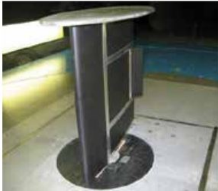
Figure 1.8: Wind tunnel testing of fix wing with PAM powered trailing edge flap actuation by Kothera and Wereley. [8]
