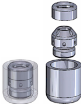
Figure 4.16: Fold-over end fitting design.
