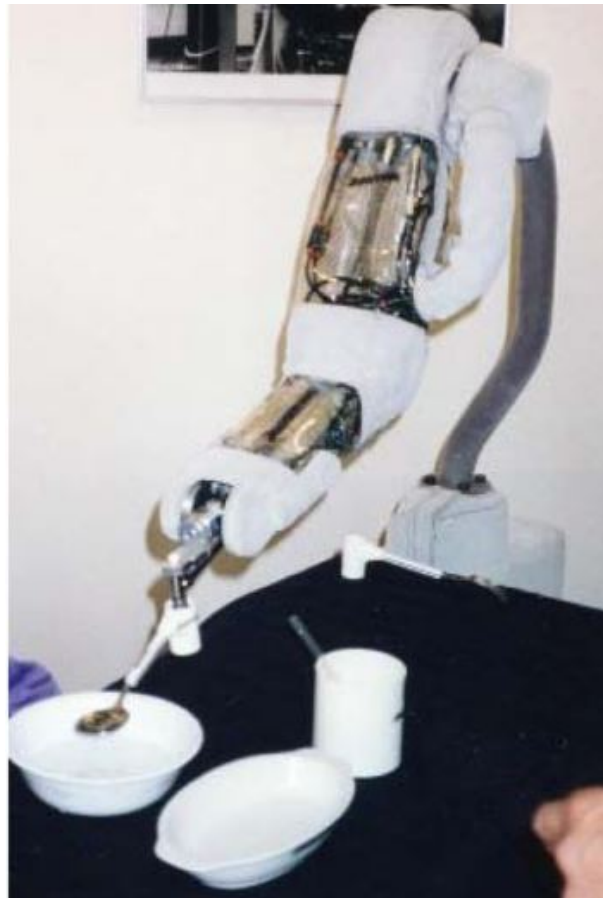
Figure 1.3: Robotic arm driven by rubbertuators. Designed by Bridgestone. From Tondur. [3]
