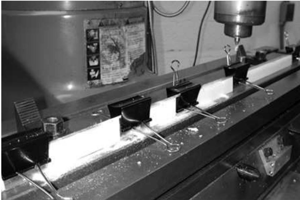
Figure 4.9: Milling leading edge slots in the fore foam core
