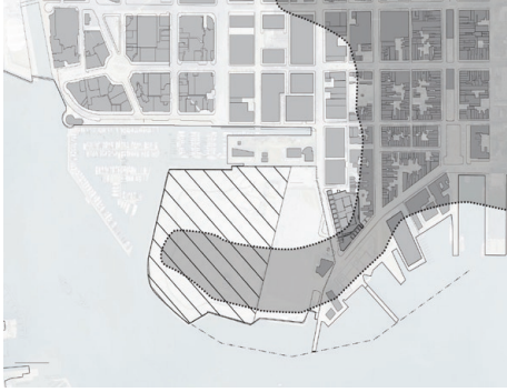
figure 29: The multimedia cap extents (hatch) covers only 2/3 of the site. the dashed, grey tone shows the sites original shape and size.
