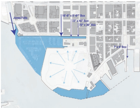
figure 30: site hydrology. The site's topography results in drainage patterns in which all water is shed from the center and towards the edges. Three wastewater outlets empty into the canal north of the site. The Jones Falls re-emerges from under a highway and flows directly west of Harbor East.
