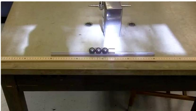
If we think of this as a collision between the two mechanical objects, it is a *super-elastic collision*, that is, the kinetic energy of the two objects after the collision is greater than the kinetic energy of the two objects before the collision. Where did the energy come from? Tell the story of the collision, walking us through what happens describing carefully the forces and energies involved so that we understand the source of the kinetic energy of ball 3 at the end of the video.
