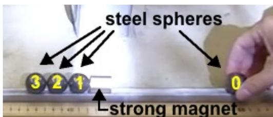
**Figure 4.5.** The Gauss gun.
