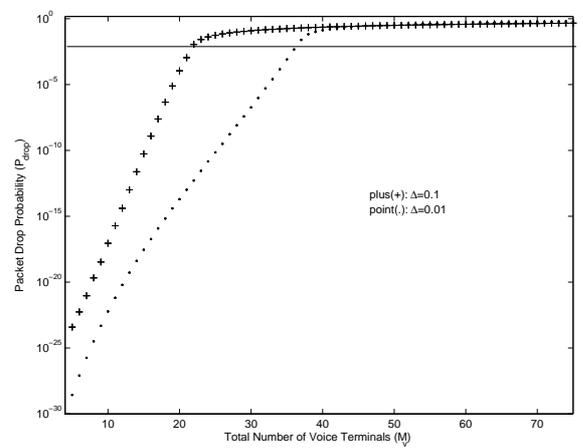
Figure 3.14: Bifurcation diagram for packet drop probability with control ( $\Delta = 0.1$ ,  $\Delta = 0.01$ ,  $\alpha = 0.0532$ ,  $\beta = \xi = 1$ )
