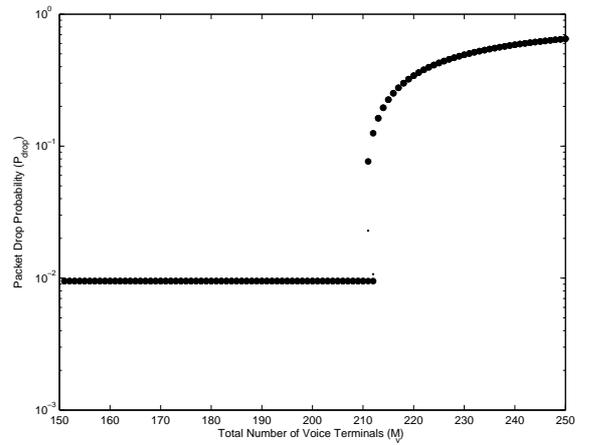
Figure 5.2: Bifurcation diagram for the packet drop probability with PBBC ( $\alpha = 0.35$ ,  $\xi = 1$ ,  $M_v$  is bifurcation parameter)
