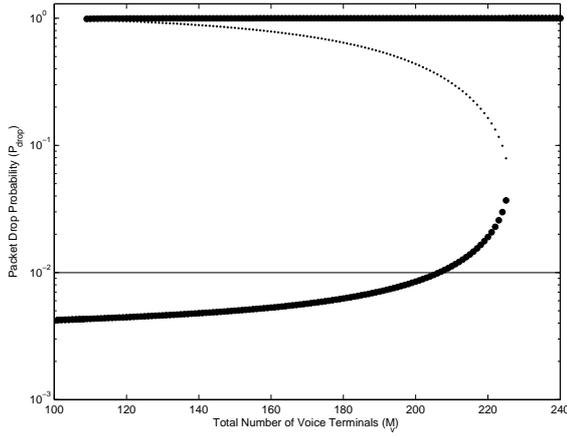
Figure 5.7: Bifurcation diagram for packet drop probability with no control ( $p = 1$ ,  $M_d = 100$ ,  $M_v$  is bifurcation parameter)
