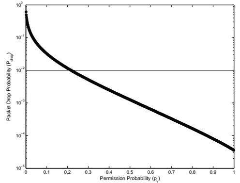
Figure 2.20: Bifurcation diagram for packet drop probability at equilibrium with power capture ( $q_1 = 0.2$  and  $q_2 = 0.8$ )
