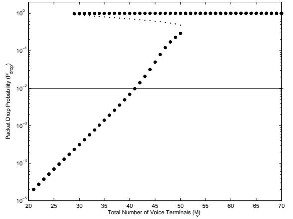
Figure 2.22: Bifurcation diagram for packet drop probability with no control ( $p_v = 0.3$ )
