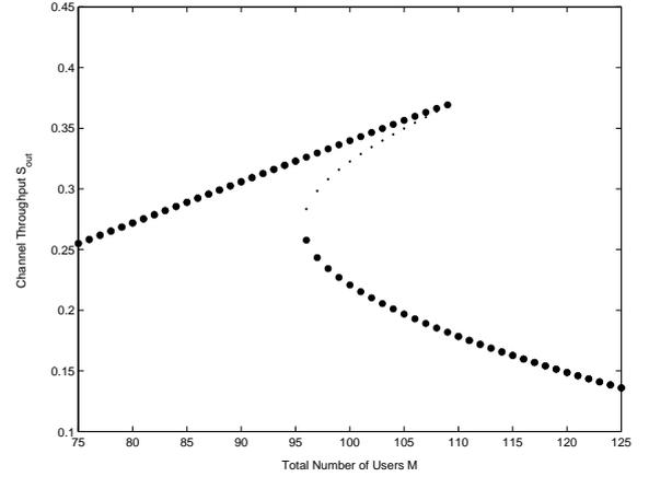
Figure 4.3: Bifurcation diagram for channel throughput ( $S_{out}$ ) when the total number of users ( $M$ ) is bifurcation parameter.  $p = 0.025$ ,  $\lambda = 0.0034$ ,  $L = 5$ .
