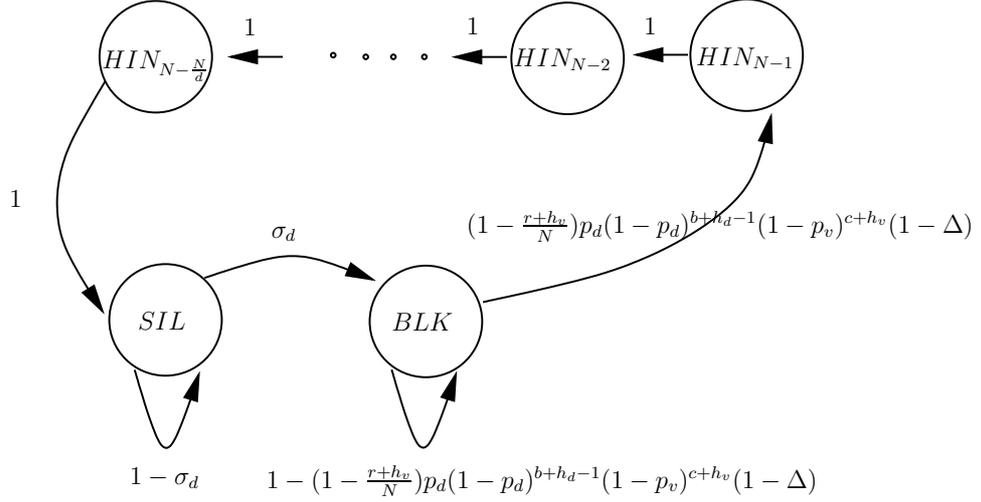
Figure 3.2: Markov Chain Model for PRMA-HS Data Subsystem over Random Packet Error Channel.
