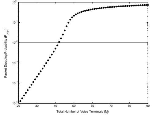
Figure 2.18: Bifurcation diagram for packet dropping probability with power capture ( $q_1 = 0.2$  and  $q_2 = 0.8$ )
