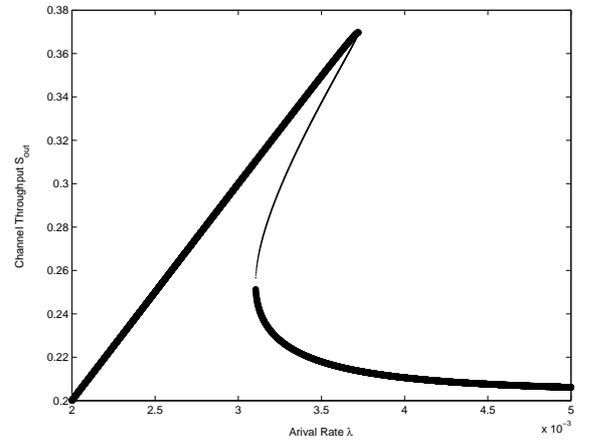
Figure 4.9: Bifurcation diagram for channel throughput ( $S_{out}$ ) when arrival rate ( $\lambda$ ) is bifurcation parameter.  $M = 100$ ,  $p = 0.025$ ,  $L = 5$ .
