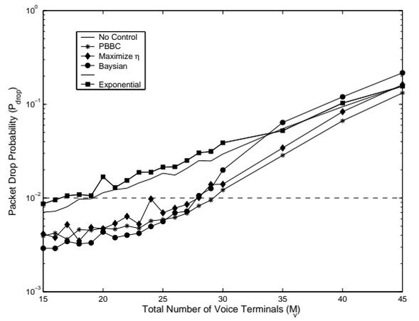
Figure 3.20: Simulation results for PRMA-HS voice+data system with delay of 10 time slot
