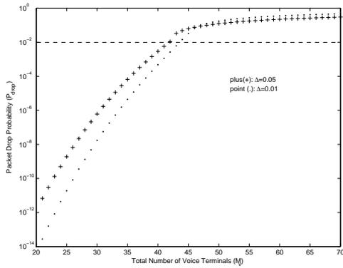
Figure 2.17: Bifurcation diagram for packet drop probability with state estimation control (minimizing  $P_{drop}$ ) ( $\Delta = 0.05$  and  $\Delta = 0.01$ )
