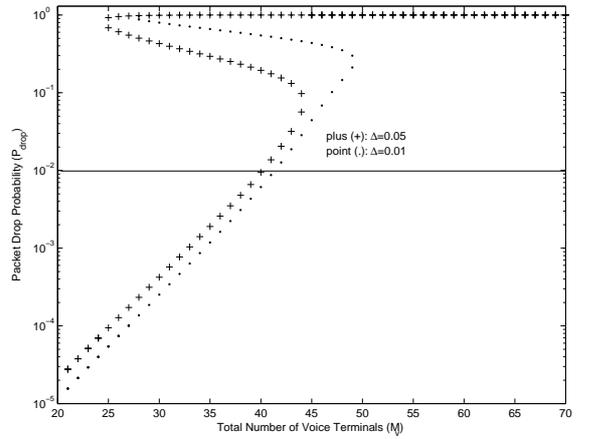
Figure 2.14: Bifurcation diagram for packet drop probability with no control ( $p_v = 0.3$  and two different values of  $\Delta$ )
