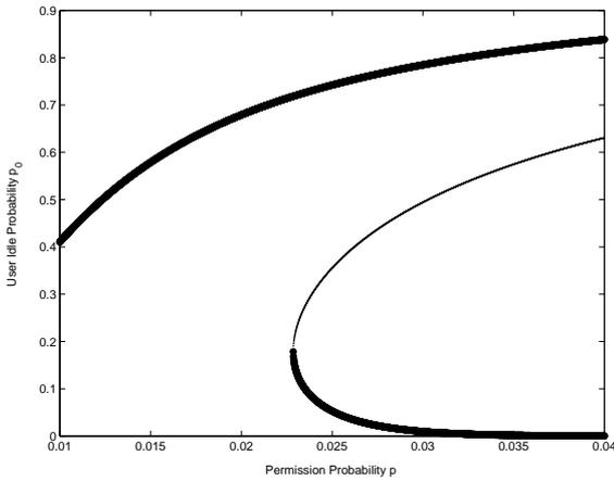
Figure 4.4: Bifurcation diagram for user idle probability ( $p_0$ ) when permission probability ( $p$ ) is bifurcation parameter.  $M = 100$ ,  $\lambda = 0.0034$ ,  $L = 5$ .
