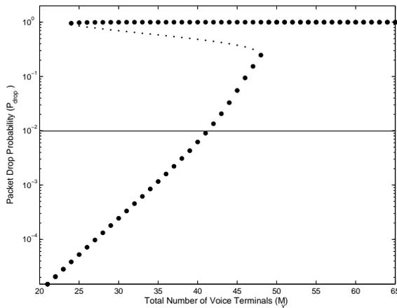
Figure 3.17: Bifurcation diagram for packet drop probability with no control ( $p_v = 0.3$ ,  $p_d = 0.044$ ,  $M_d = 36$ ,  $M_v$  bifurcation parameter,  $p_{max} = 0.9$ )
