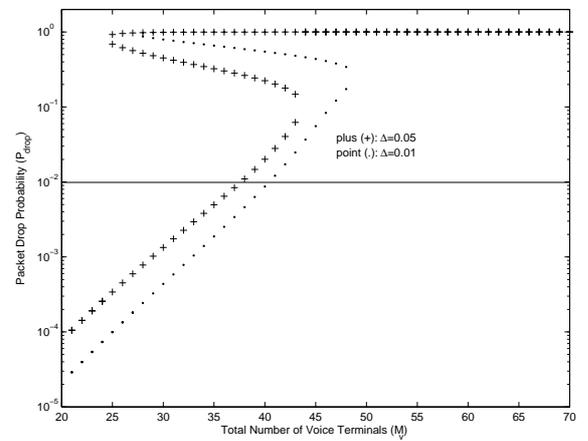
Figure 2.28: Bifurcation diagram for packet drop probability with no control ( $p_v = 0.3$  and two different values for  $\Delta$ )
