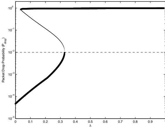
Figure 2.13: Bifurcation diagram for packet drop probability with no control ( $\Delta$  is bifurcation parameter,  $p_v = 0.3$ ,  $M_v = 25$ )
