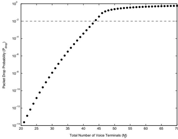
Figure 3.11: Bifurcation diagram for packet drop probability with state estimation control (minimizing  $P_{drop}$ ) ( $M_v$  bifurcation parameter)
