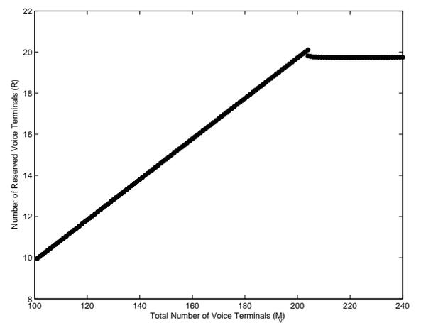
Figure 5.12: Bifurcation diagram for the number of reserved terminals with PBBC ( $\alpha = 0.35$ ,  $\xi = 1$ ,  $M_d = 100$ ,  $M_v$  is bifurcation parameter)
