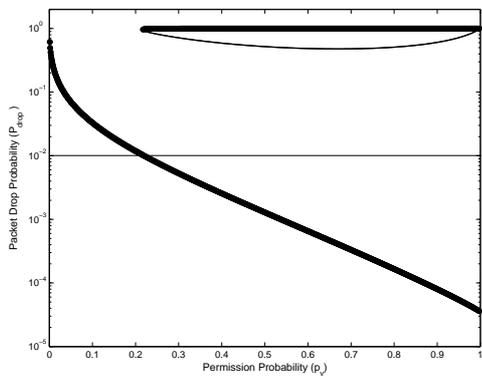
Figure 2.19: Bifurcation diagram for packet drop probability with no capture
