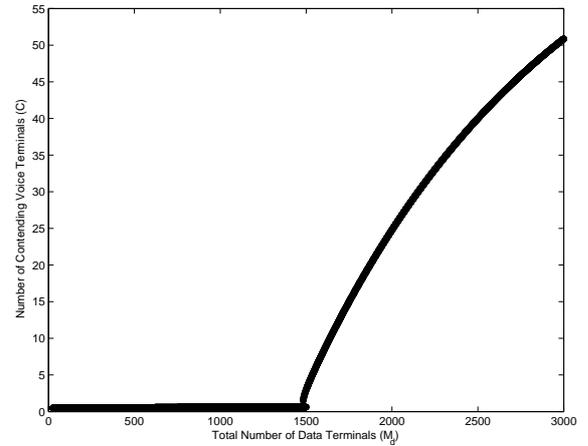
Figure 5.18: Bifurcation diagram for the number of contending terminals with PBBC ( $\alpha = 0.35$ ,  $\xi = 1$ ,  $M_v = 100$ ,  $M_d$  is bifurcation parameter)
