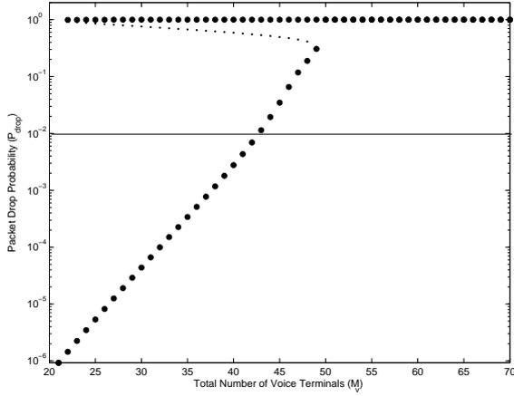
Figure 2.9: Bifurcation diagram for packet drop probability with no control ( $p_v = 0.4$ )
