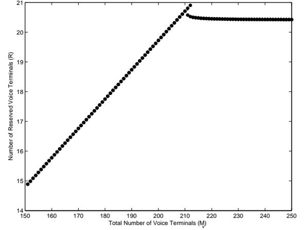
Figure 5.6: Bifurcation diagram for the number of reserved terminals with PBBC ( $\alpha = 0.35$ ,  $\xi = 1$ ,  $M_v$  is bifurcation parameter)
