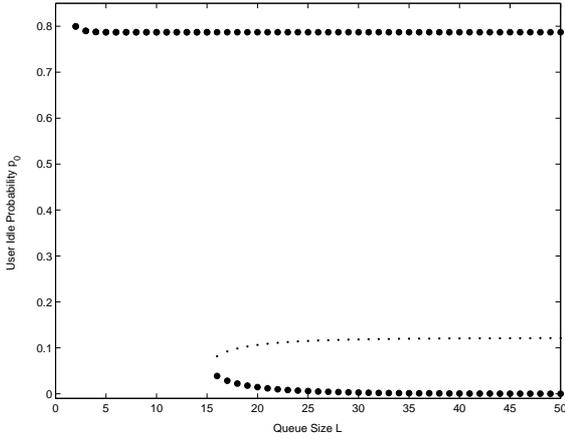
Figure 4.6: Bifurcation diagram for user idle probability ( $p_0$ ) when queue size ( $L$ ) is bifurcation parameter.  $M = 100$ ,  $\lambda = 0.0034$ ,  $p = 0.025$ .
