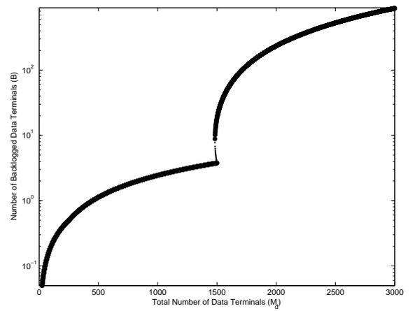
Figure 5.22: Bifurcation diagram for the number of backlogged data terminals with PBBC ( $\alpha = 0.35$ ,  $\xi = 1$ ,  $M_v = 100$ ,  $M_d$  is bifurcation parameter)
