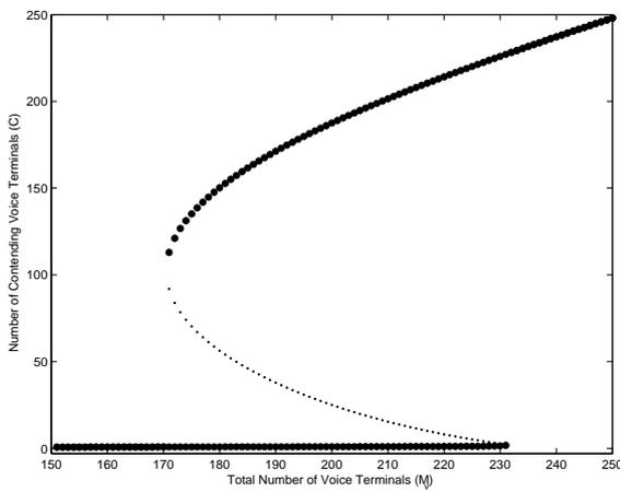
Figure 5.3: Bifurcation diagram for the number of contending terminals with no control ( $p_v = 1$  and  $M_v$  is bifurcation parameter)
