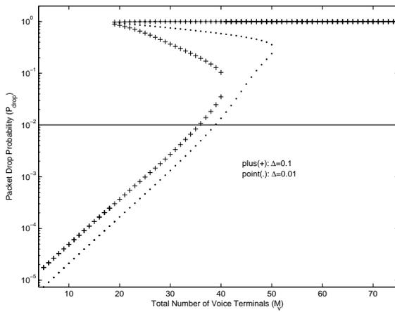
Figure 3.13: Bifurcation diagram for packet drop probability with no control ( $p = 0.2$  and two different values for  $\Delta$ )
