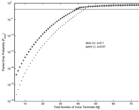
Figure 3.15: Bifurcation diagram for packet drop probability with state estimation control (maximizing throughput) ( $\Delta = 0.1$ ,  $\Delta = 0.01$ ,  $M_v$  bifurcation parameter,  $p_{max} = 0.9$ )
