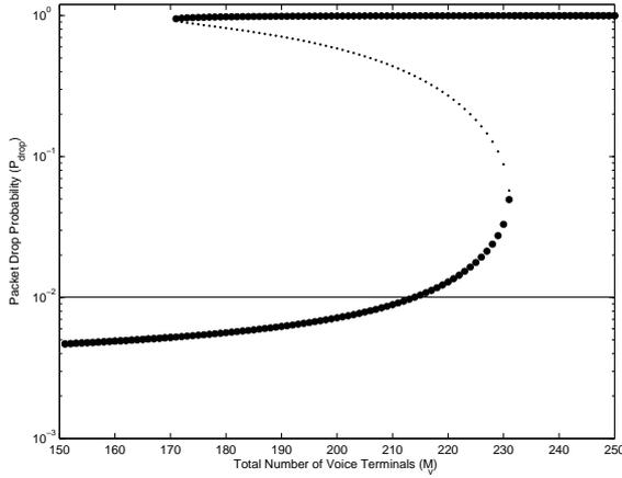
Figure 5.1: Bifurcation diagram for packet drop probability with no control ( $p_v = 1$  and  $M_v$  is bifurcation parameter)
