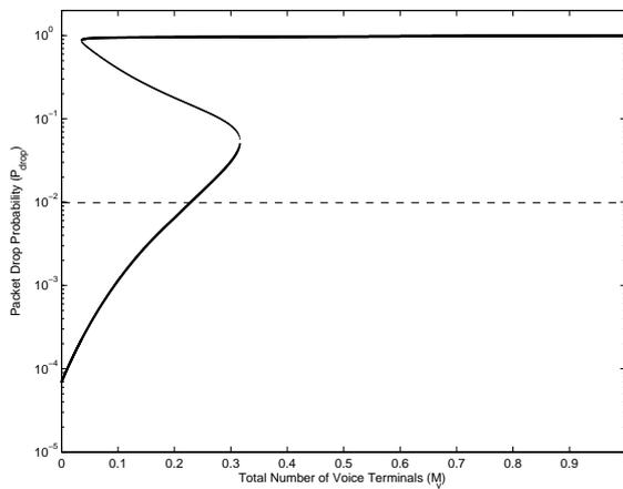
Figure 2.27: Bifurcation diagram for packet drop probability no control ( $\Delta$  is bifurcation parameter,  $p_v = 0.3$ ,  $M_v = 25$ )
