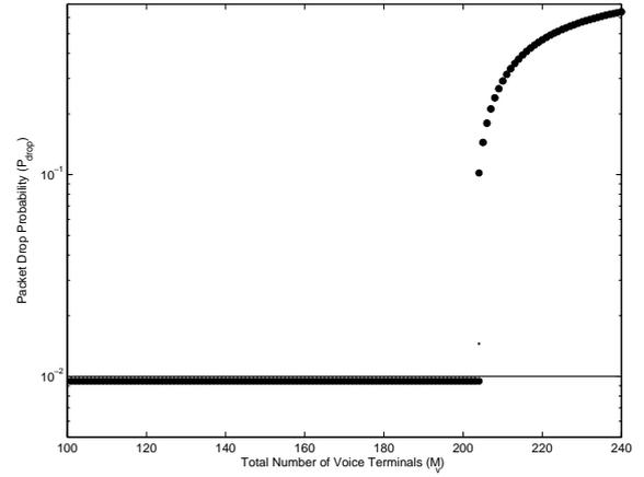
Figure 5.8: Bifurcation diagram for the packet drop probability with PBBC ( $\alpha = 0.35$ ,  $\xi = 1$ ,  $M_d = 100$ ,  $M_v$  is bifurcation parameter)
