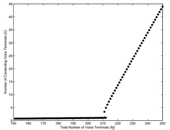
Figure 5.4: Bifurcation diagram for the number of contending terminals with PBBC ( $\alpha = 0.35$ ,  $\xi = 1$ ,  $M_v$  is bifurcation parameter)
