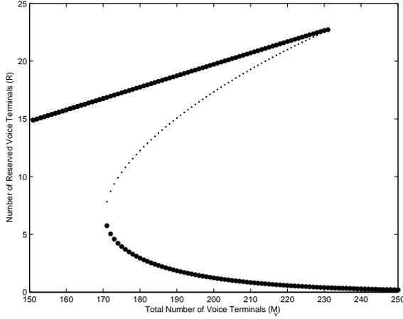
Figure 5.5: Bifurcation diagram for the number of reserved terminals with no control ( $p_v = 1$  and  $M_v$  is bifurcation parameter)
