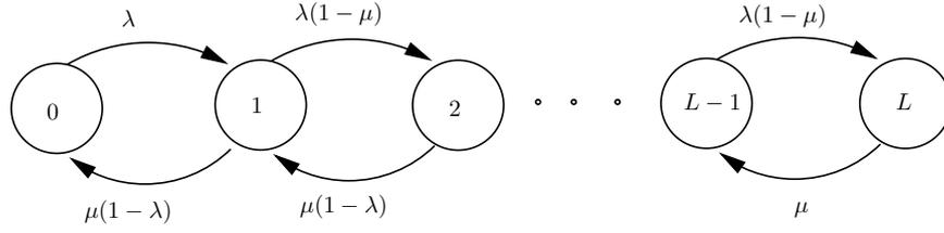
Figure 4.1: Probability flow chart of the buffer.
