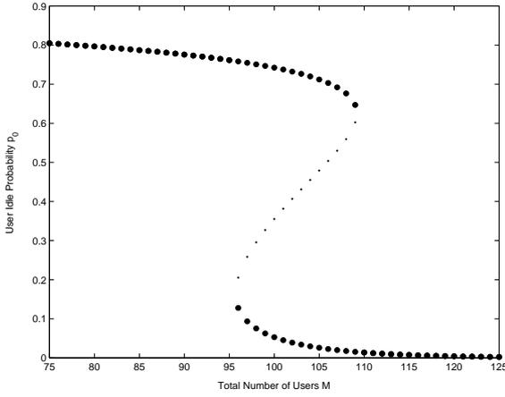
Figure 4.2: Bifurcation diagram for user idle probability ( $p_0$ ) when the total number of users ( $M$ ) is bifurcation parameter.  $p = 0.025$ ,  $\lambda = 0.0034$ ,  $L = 5$ .
