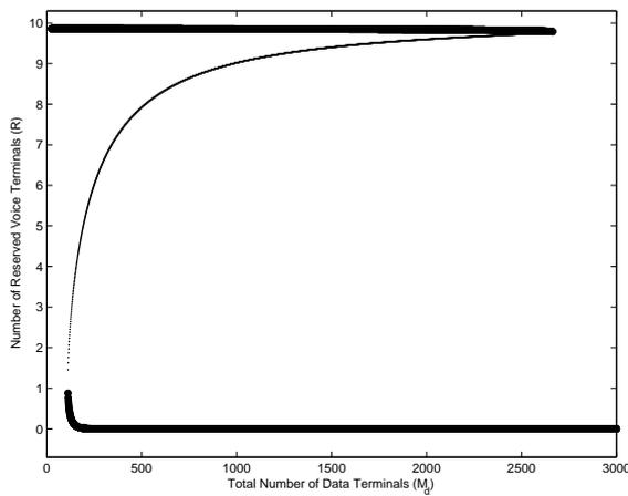
Figure 5.19: Bifurcation diagram for the number of reserved terminals with no control ( $p = 1$ ,  $M_v = 100$ ,  $M_d$  is bifurcation parameter)
