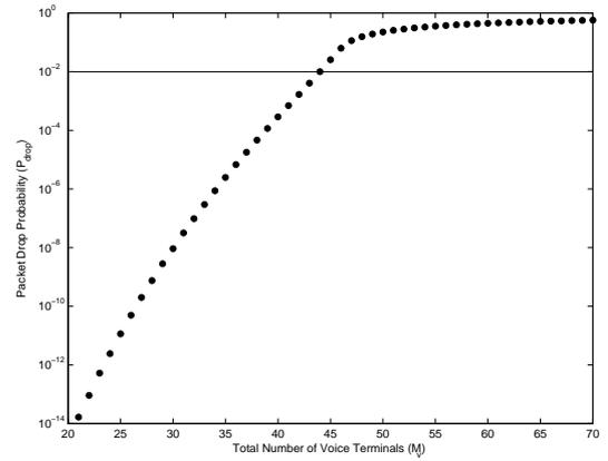
Figure 2.26: Bifurcation diagram for packet drop probability with state estimation control (minimizing  $P_{drop}$ )
