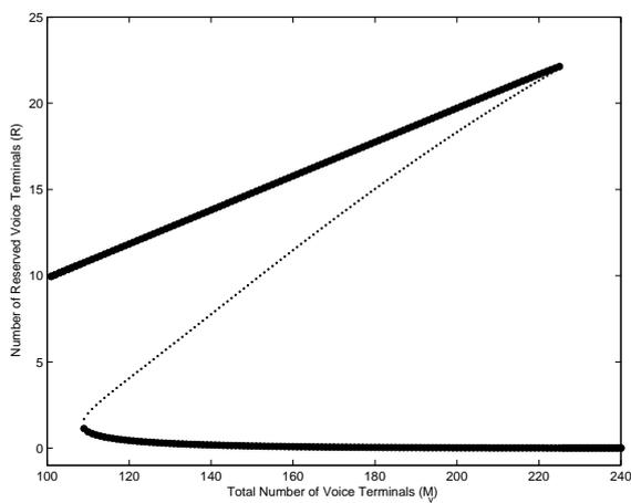
Figure 5.11: Bifurcation diagram for the number of reserved terminals with no control ( $p = 1$ ,  $M_d = 100$ ,  $M_v$  is bifurcation parameter)
