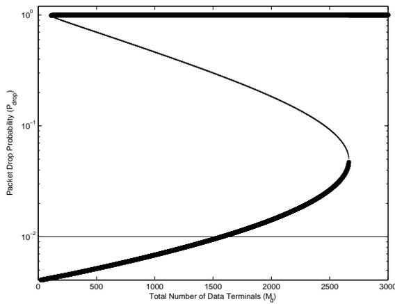
Figure 5.15: Bifurcation diagram for packet drop probability with no control ( $p = 1$ ,  $M_v = 100$ ,  $M_d$  is bifurcation parameter)
