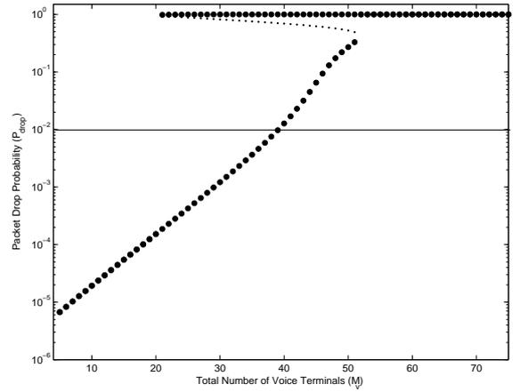
Figure 3.4: Bifurcation diagram for the packet drop probability with no control ( $p = 0.2$  and  $M_v$  is bifurcation parameter)
