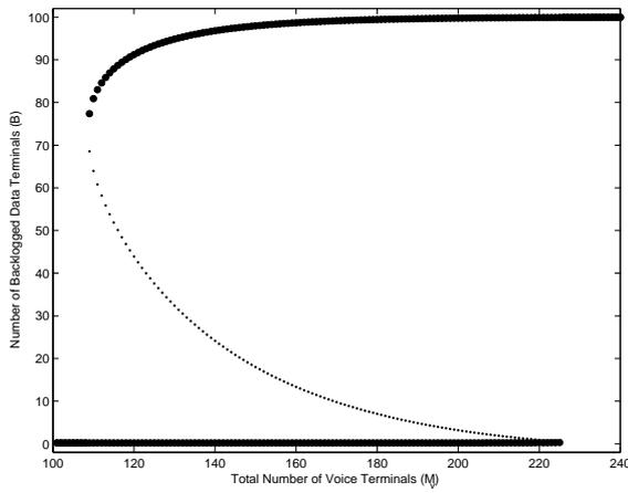
Figure 5.13: Bifurcation diagram for the number of backlogged data terminals with no control ( $p = 1$ ,  $M_d = 100$ ,  $M_v$  is bifurcation parameter)
