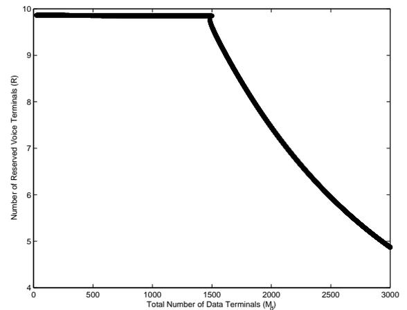
Figure 5.20: Bifurcation diagram for the number of reserved terminals with PBBC ( $\alpha = 0.35$ ,  $\xi = 1$ ,  $M_v = 100$ ,  $M_d$  is bifurcation parameter)
