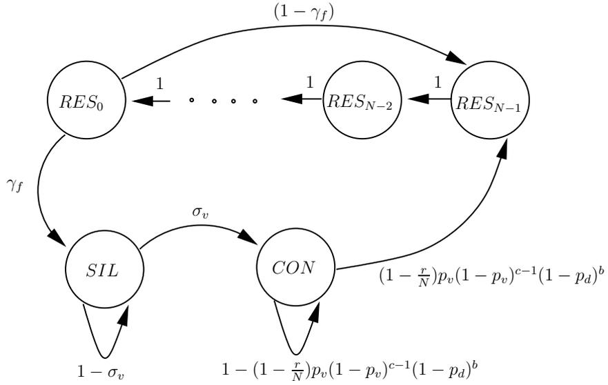
Figure 1.1: Markov chain model for PRMA voice subsystem.
