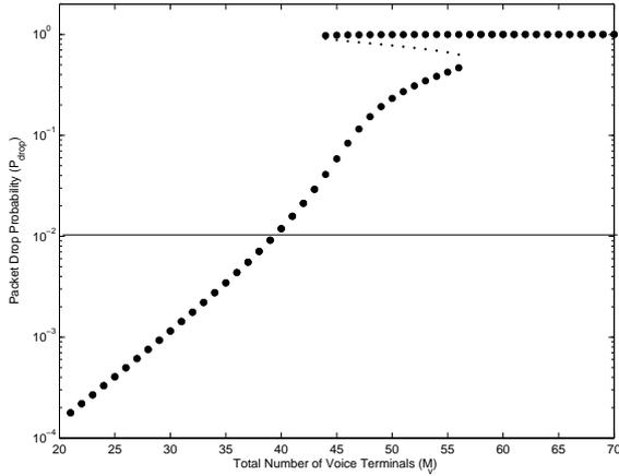
Figure 2.7: Bifurcation diagram for packet drop probability with no control ( $p_v = 0.2$ )
