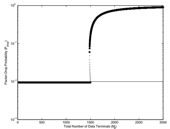
Figure 5.16: Bifurcation diagram for the packet drop probability with PBBC ( $\alpha = 0.35$ ,  $\xi = 1$ ,  $M_v = 100$ ,  $M_d$  is bifurcation parameter)
