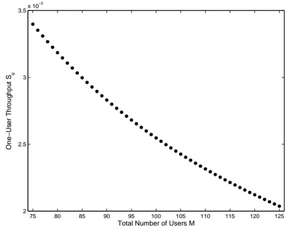
Figure 4.12: Bifurcation diagram for channel throughput ( $S_u$ ) with price based bifurcation, the total number of users ( $M$ ) bifurcation parameter,  $\lambda = 0.0034$ , and  $L = 5$ .
