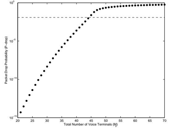
Figure 2.12: Bifurcation diagram for packet drop probability with state estimation control (minimizing  $P_{drop}$ )
