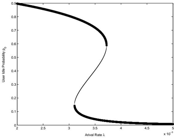
Figure 4.8: Bifurcation diagram for user idle probability ( $p_0$ ) when arrival rate ( $\lambda$ ) is bifurcation parameter.  $M = 100$ ,  $p = 0.025$ ,  $L = 5$ .
