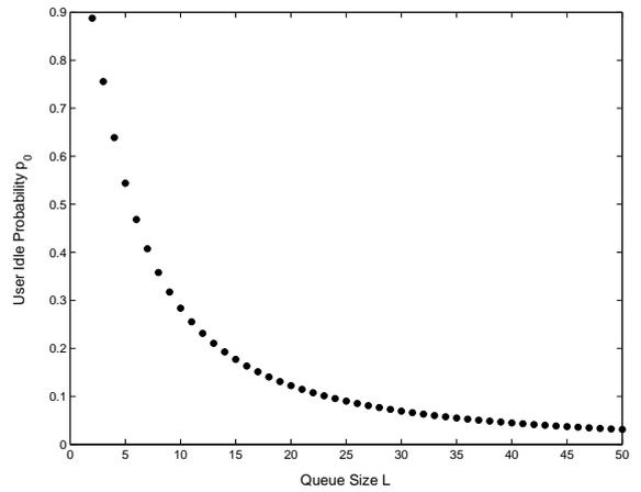
Figure 4.14: Bifurcation diagram for user idle probability ( $p_0$ ) with price based bifurcation, queue size ( $L$ ) bifurcation parameter,  $\lambda = 0.0034$ , and  $M = 100$ .
