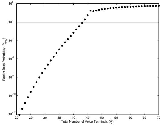
Figure 2.25: Bifurcation diagram for packet drop probability with state estimation control (maximizing throughput)
