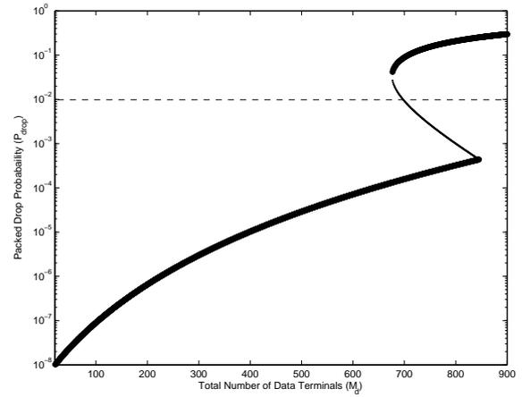
Figure 3.12: Bifurcation diagram for packet drop probability with state estimation control (minimizing  $P_{drop}$ ) ( $M_d$  bifurcation parameter)
