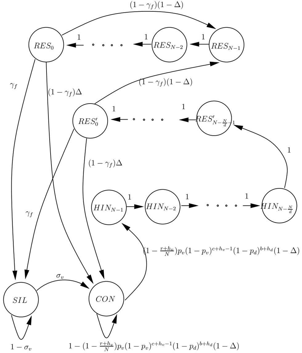
Figure 3.1: Markov Chain Model for PRMA-HS Voice Subsystem over Random Packet Error Channel.
