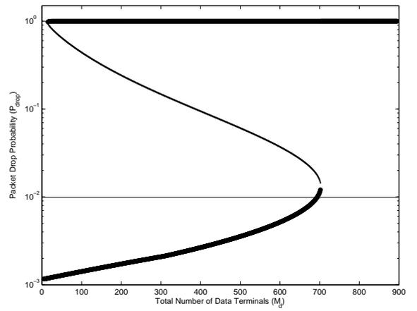
Figure 3.6: Bifurcation diagram for the packet drop probability with no control ( $p = 0.2$  and  $M_d$  is bifurcation parameter)
