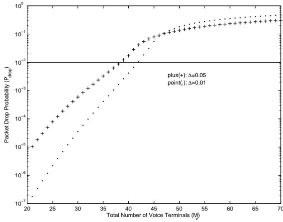
Figure 2.29: Bifurcation diagram for packet drop probability with control ( $\Delta = 0.05$ ,  $\Delta = 0.01$ ,  $\alpha = 1.04$ ,  $\beta = \xi = 1$ )
