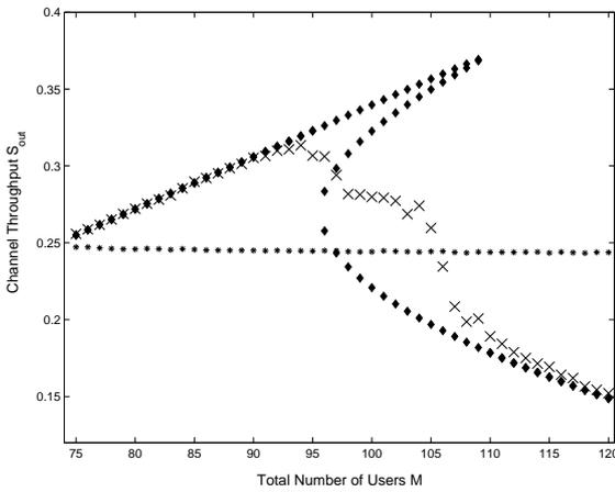
Figure 4.13: Analytical vs. Simulation - Diamonds are analytical results (solutions to equilibrium equations) and Crosses are simulation results
