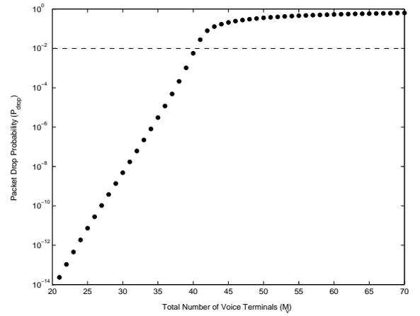
Figure 2.10: Bifurcation diagram for packet drop probability with the price based control ( $\alpha = 0.114, \beta = \xi = 1$ )
