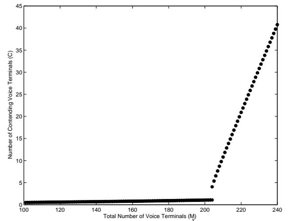
Figure 5.10: Bifurcation diagram for the number of contending terminals with PBBC ( $\alpha = 0.35$ ,  $\xi = 1$ ,  $M_d = 100$ ,  $M_v$  is bifurcation parameter)
