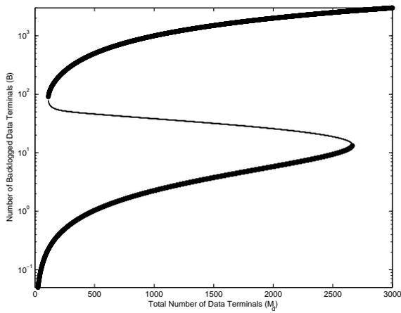
Figure 5.21: Bifurcation diagram for the number of backlogged data terminals with no control ( $p = 1$ ,  $M_v = 100$ ,  $M_d$  is bifurcation parameter)
