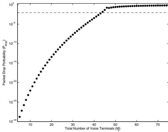
Figure 3.9: Bifurcation diagram for packet drop probability with state estimation control (maximizing throughput) ( $p_{max} = 0.9$  and  $M_v$  bifurcation parameter)
