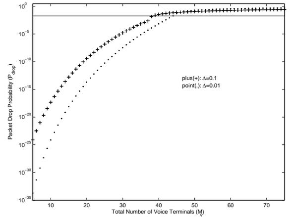
Figure 3.16: Bifurcation diagram for packet drop probability with state estimation control (minimizing  $P_{drop}$ ) ( $\Delta = 0.1$ ,  $\Delta = 0.01$ ,  $M_v$  bifurcation parameter)
