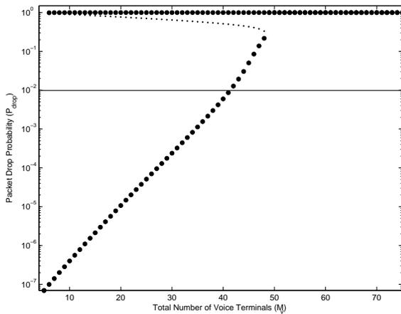
Figure 3.5: Bifurcation diagram for packet drop probability with no control ( $p = 0.3$  and  $M_v$  is bifurcation parameter)
