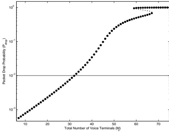
Figure 3.3: Bifurcation diagram for packet drop probability with no control ( $p = 0.1$  and  $M_v$  is bifurcation parameter)
