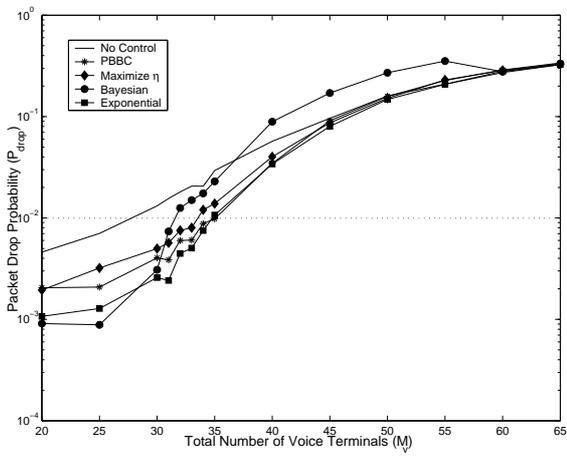
Figure 3.19: Simulation results for PRMA-HS voice+data system with delay of 1 time slot
