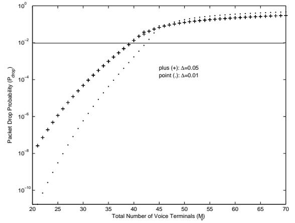
Figure 2.30: Bifurcation diagram for packet drop probability with state observation control (maximizing throughput) ( $\Delta = 0.05$  and  $\Delta = 0.01$ )
