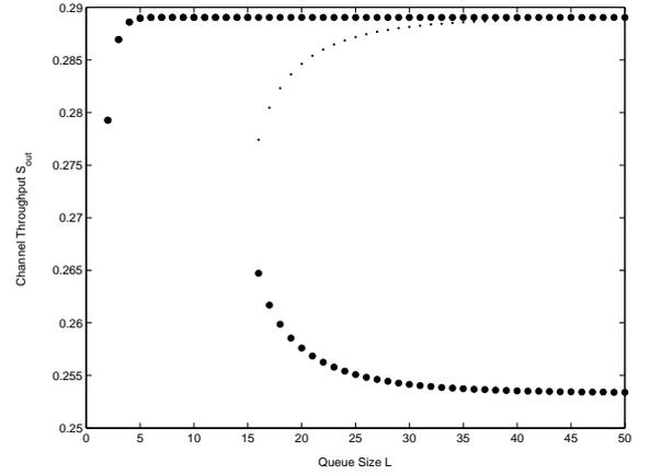
Figure 4.7: Bifurcation diagram for channel throughput ( $S_{out}$ ) when queue size ( $L$ ) is bifurcation parameter.  $M = 100$ ,  $\lambda = 0.0034$ ,  $p = 0.025$ .
