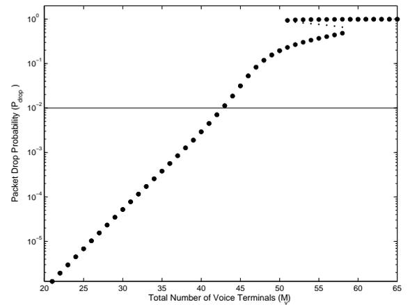
Figure 3.18: Bifurcation diagram for packet drop probability with capture effect ( $q_1 = q_2 = 0.5$ )
