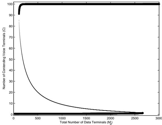
Figure 5.17: Bifurcation diagram for the number of contending terminals with no control ( $p = 1$ ,  $M_v = 100$ ,  $M_d$  is bifurcation parameter)
