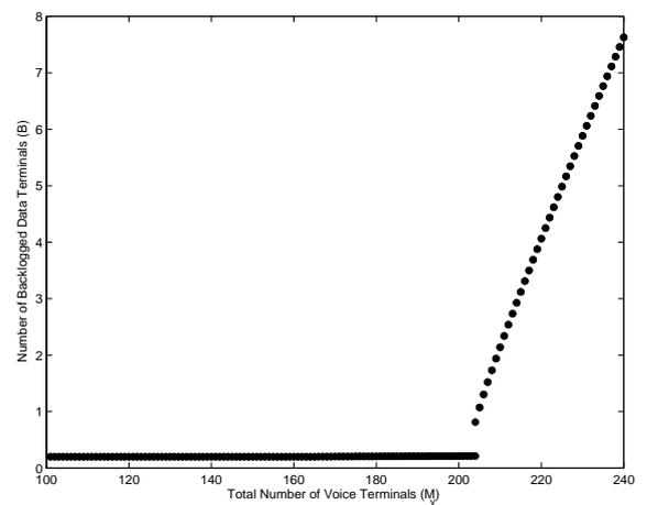
Figure 5.14: Bifurcation diagram for the number of backlogged data terminals with PBBC ( $\alpha = 0.35$ ,  $\xi = 1$ ,  $M_d = 100$ ,  $M_v$  is bifurcation parameter)
