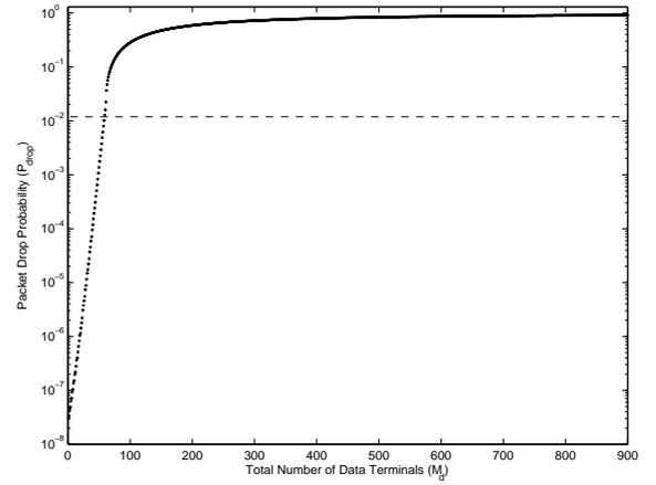
Figure 3.8: Bifurcation diagram for packet drop probability with the price based bifurcation control ( $\alpha = 0.0644$ ,  $\beta = \xi = 1$ ,  $M_d$  bifurcation parameter)
