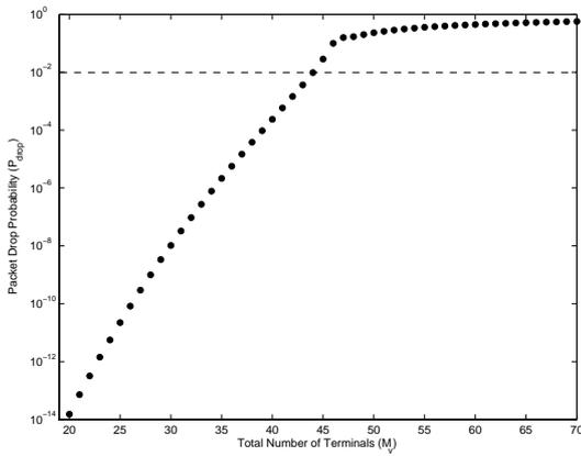
Figure 2.11: Bifurcation diagram for packet drop probability with state estimation control (maximizing throughput) ( $p_{v_{max}} = 0.9$ )
