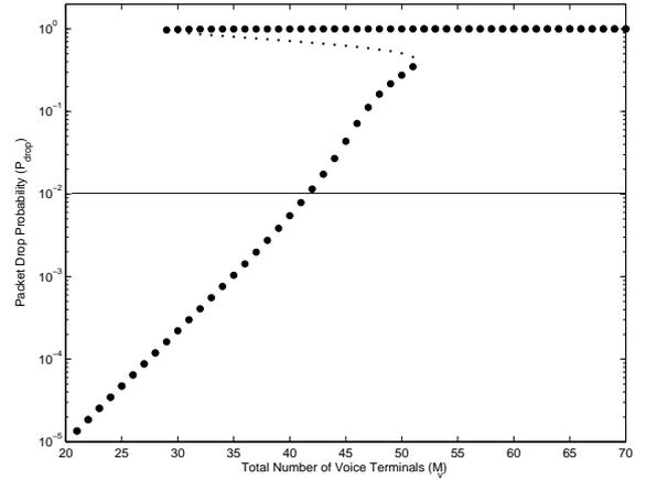
Figure 2.8: Bifurcation diagram for packet drop probability with no control ( $p_v = 0.3$ )
