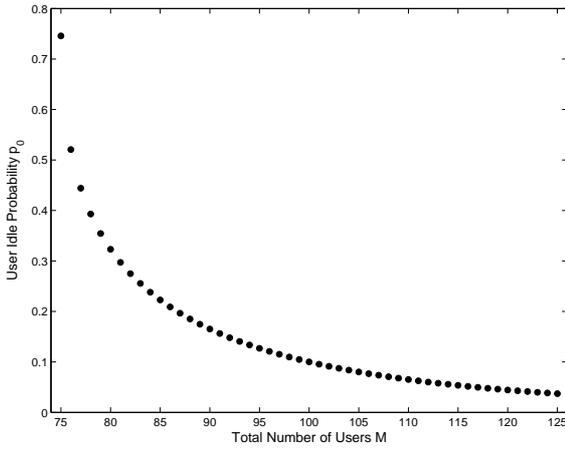
Figure 4.11: Bifurcation diagram for user idle probability ( $p_0$ ) with price based bifurcation, the total number of users ( $M$ ) bifurcation parameter,  $\lambda = 0.0034$ , and  $L = 5$ .
